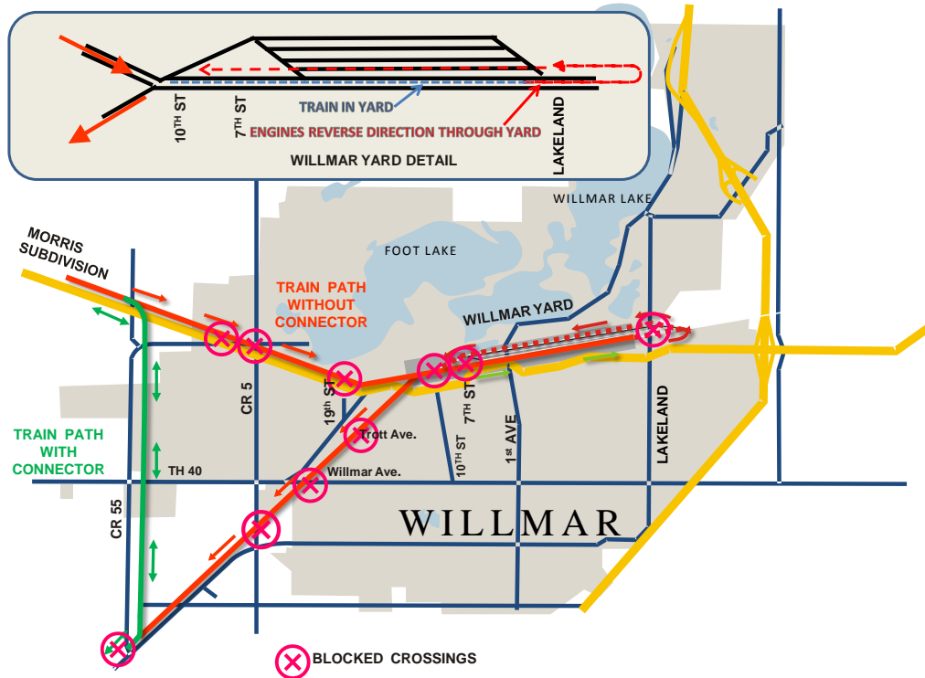
Exhibit 2: Map Illustrating Train Movement Required to Switch from the Morris to the Marshall Subdivisions
