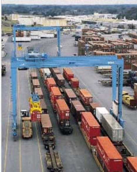
Figure 6: Small Multi-track terminal with Rubber Tired Gantries (RTG's or rolling cranes)
