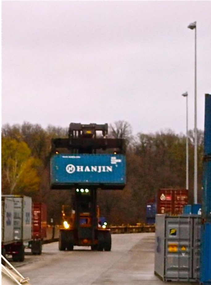
Figure 5: Small Multi-track Container Terminal with Reach Stackers
