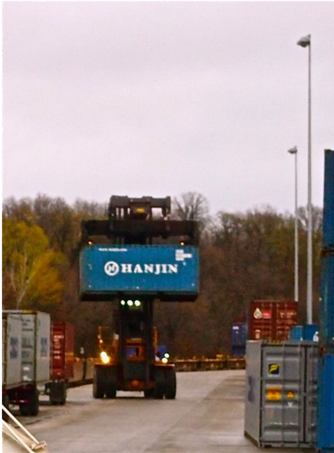
Figure 4: Container Top Handler Loading Double Stack Cars
