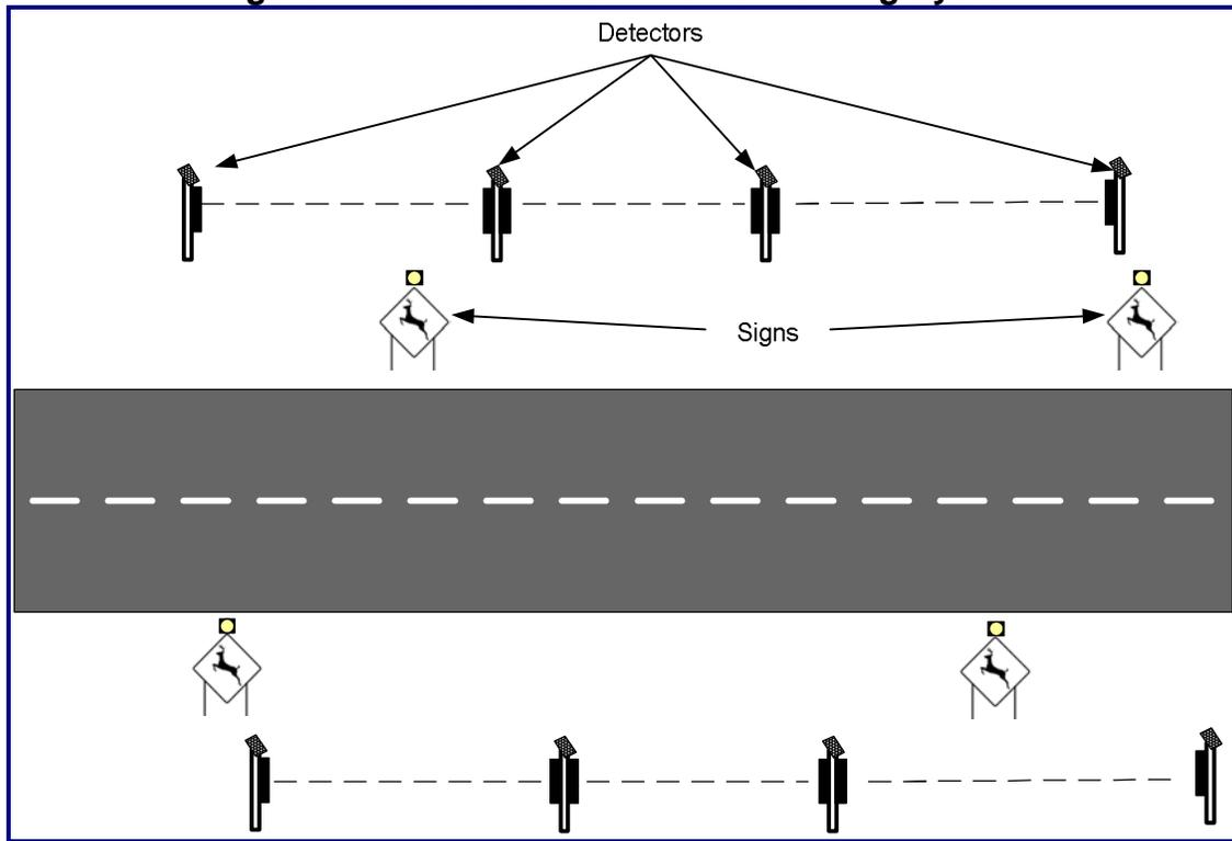
Since this is a system that requires periodic inspection and maintenance, support from the Mn/DOT District will be a key factor in ensuring its success. Site selection is also an important part of implementation. High concentrations of wildlife movement are needed to make a detection system cost effective, as the total system cost will scale with the number of feet of roadway to be covered. A short list of the steps involved with deploying such a system is provided below.
