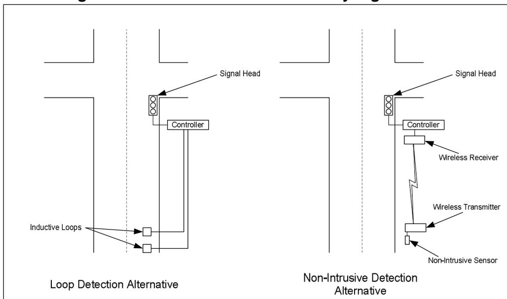
Deployment of truck priority signal systems should be approached on a corridor basis, which will involve the assessment of current signal hardware in multiple jurisdictions. All modern intersection signal controllers support a priority function, but there may be cases where older systems are still in use.
