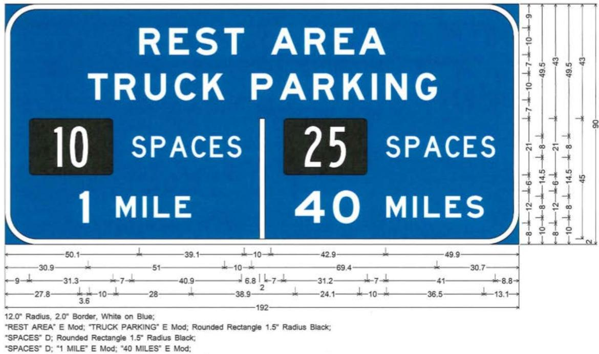
Figure B.2. Hybrid CMS design for displaying truck parking information for two downstream rest areas, with overall dimensions of 7.5 x 16 feet (2.3 x 4.9 m).
