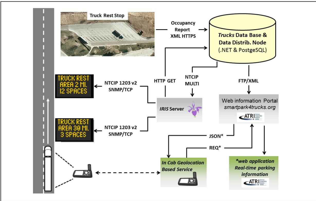
Figure 5.7. System architecture for archiving and disseminating truck parking information
