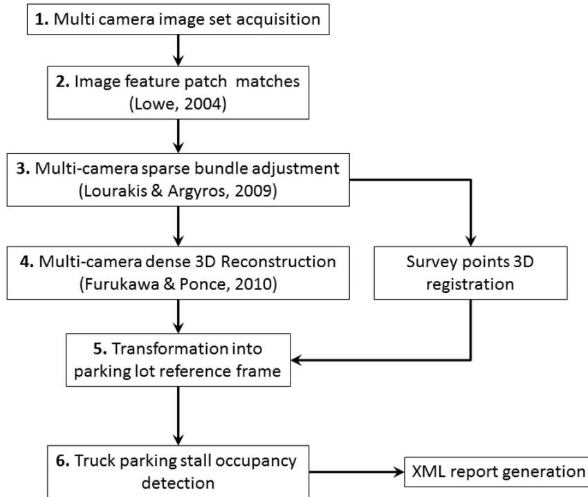
Figure 3.1. Algorithm steps for truck parking space occupancy detection.
