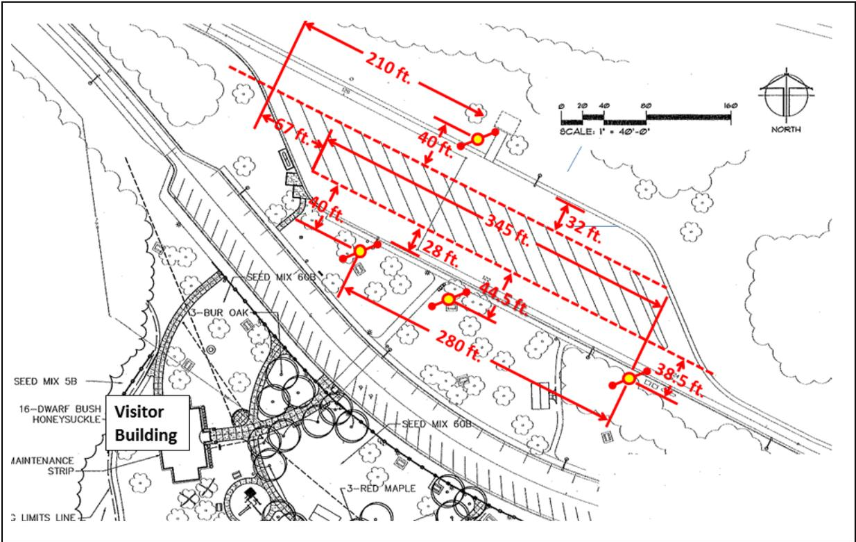
Figure 5.5. Enfield truck parking camera system site plan.
