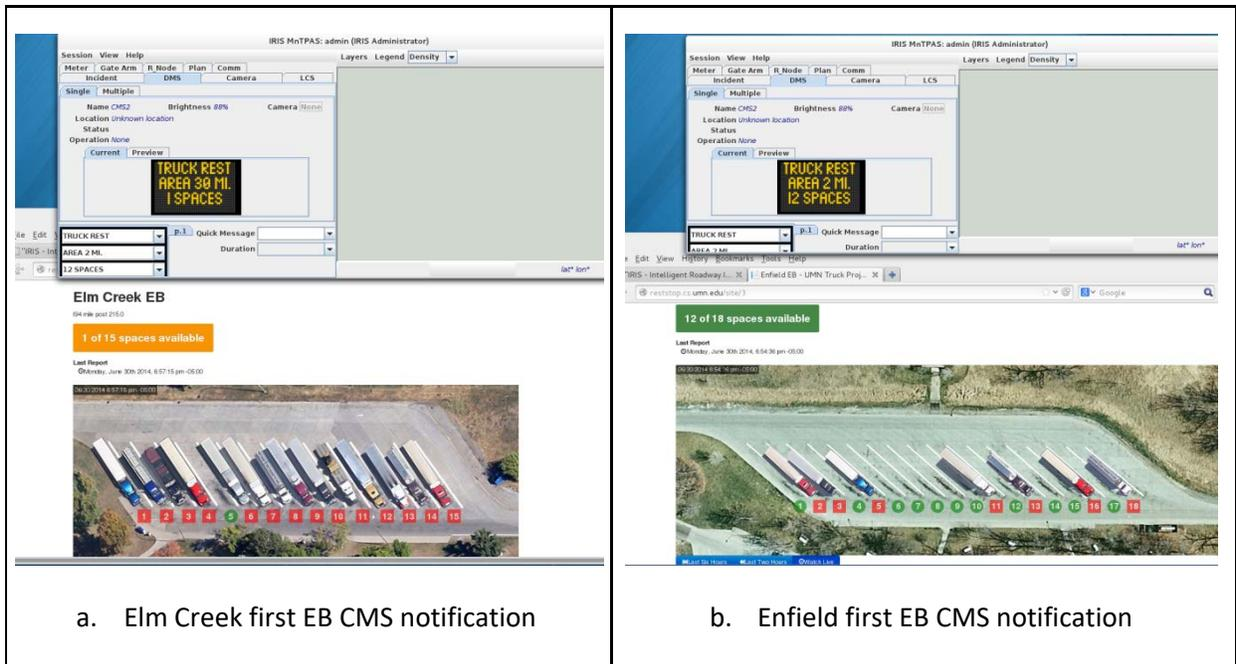
Figure 7.2. CMS verification of parking status shown through IRIS and TPAS DDS interfaces.
