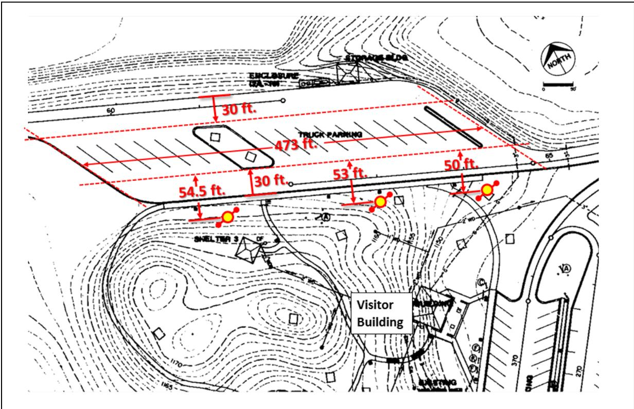
Figure 5.3. Big Spunk Lake camera system site plan.
