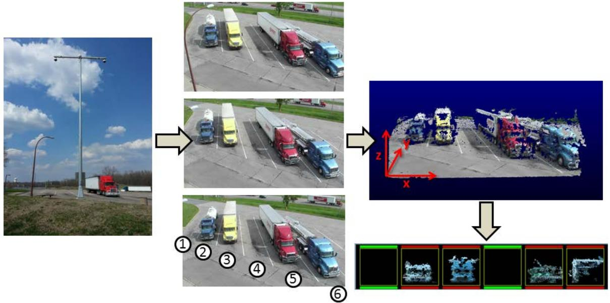
Figure 3.2. Truck 3D occupancy vehicle detection for a group of parking spaces.
