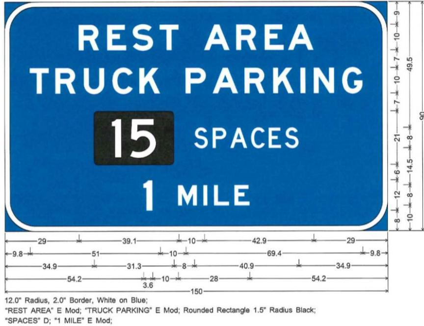
Figure B.1. Hybrid single rest area downstream truck parking information CMS design, with overall dimensions of 7.5 x 12.5 feet (2.3 x 3.8 m).
