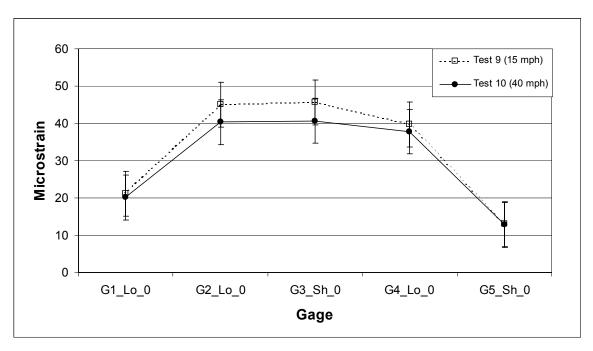
Figure 3.10 Dynamic response of bridge #04006 – Trucks 1 and 2 (measured)
