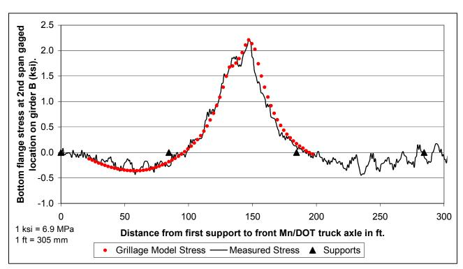
Figure 3.13 Bridge #54004 over the Red River Stress at  $2^{nd}$  span gaged location vs. Mn/DOT truck position traveling in the westbound lane
