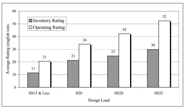
Figure 3.4 Average inventory and operating ratings for different design loads
