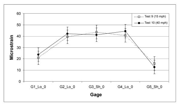
Figure 3.11 Dynamic response of bridge #04006 – Trucks 3 and 4 (measured)
