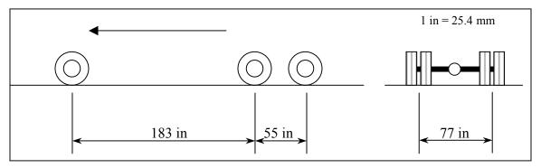
Figure 3.8 Average axle spacing of test trucks
