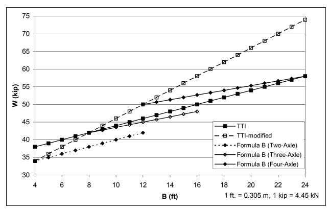
Figure 2.3 Comparison of different axle-group-weight formulas.
