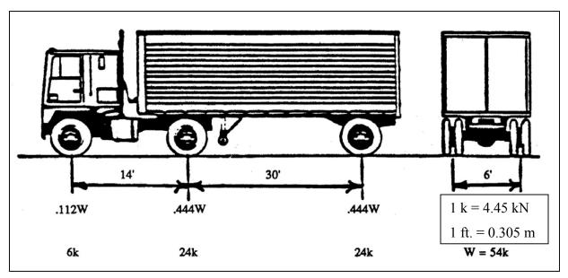
Figure 2.5 Fatigue truck. (Moses et al. 1987)
