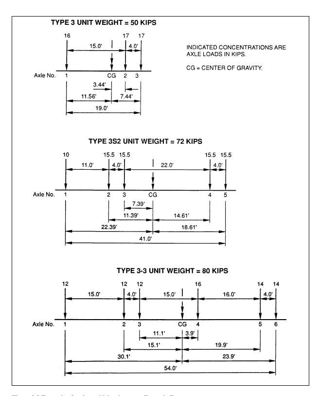
Figure 2.2 Example of rating vehicles that meet Formula B.
