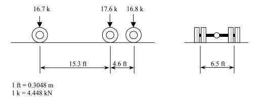
Figure 2.10 3-axle single bodied truck (test truck) (GVW = 51.1 k (227 kN))
