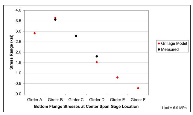
Figure 3.14 Bridge #9276, grillage analysis model and measured results for a Mn/DOT truck in the left lane
