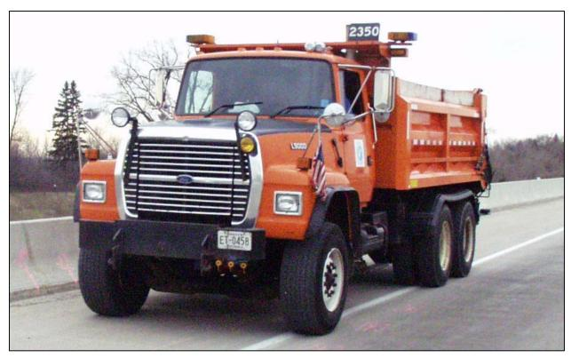
Figure 3.7 Typical 3-axle Mn/DOT truck used for live load tests
