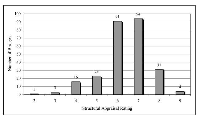
Figure 3.5 Structural valuation appraisal rating for bridges on the selected routes
