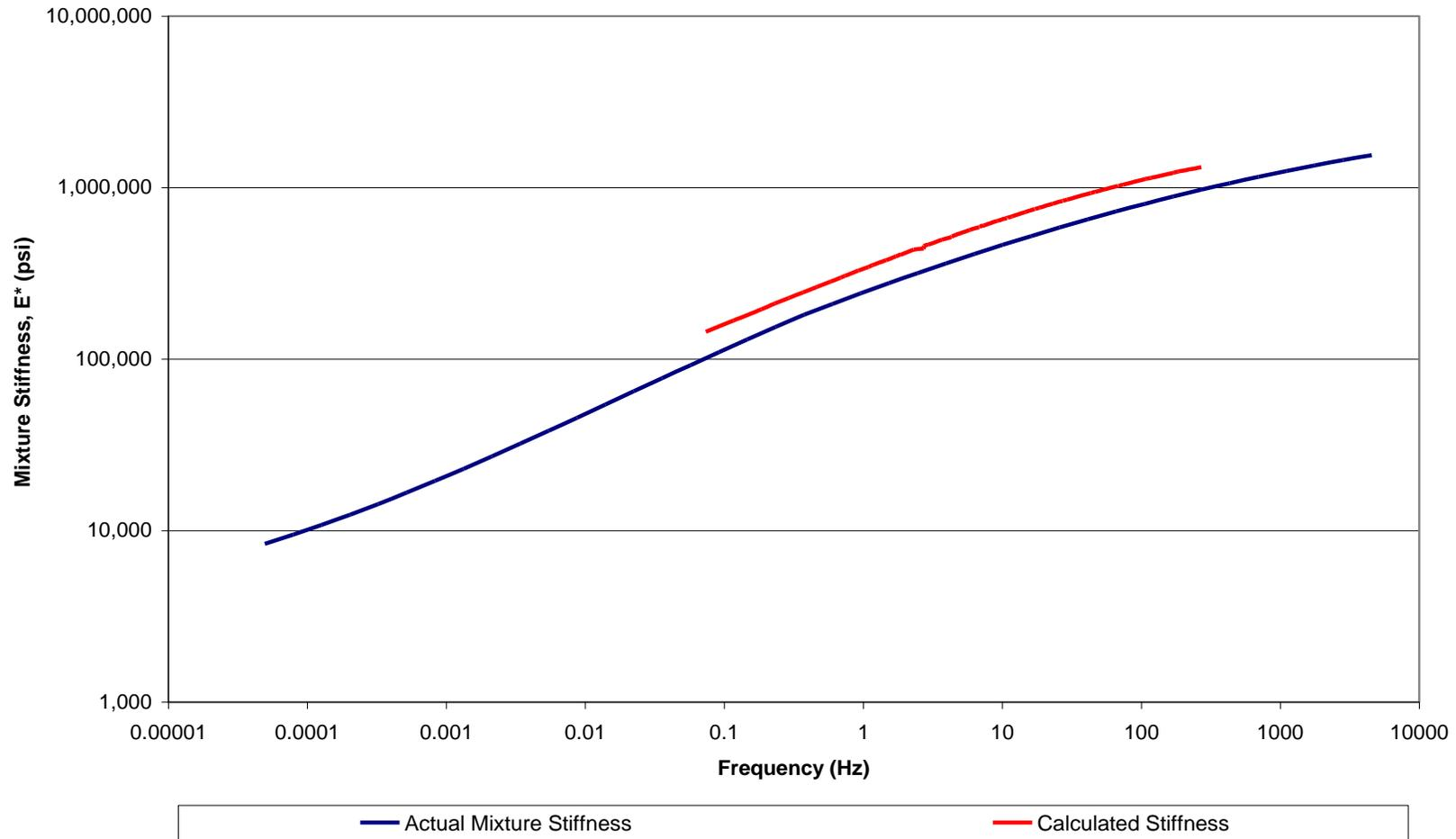
Figure 1: Measured and Predicted Stiffness Comparison ( $T_r = 20^\circ\text{C}$ )
