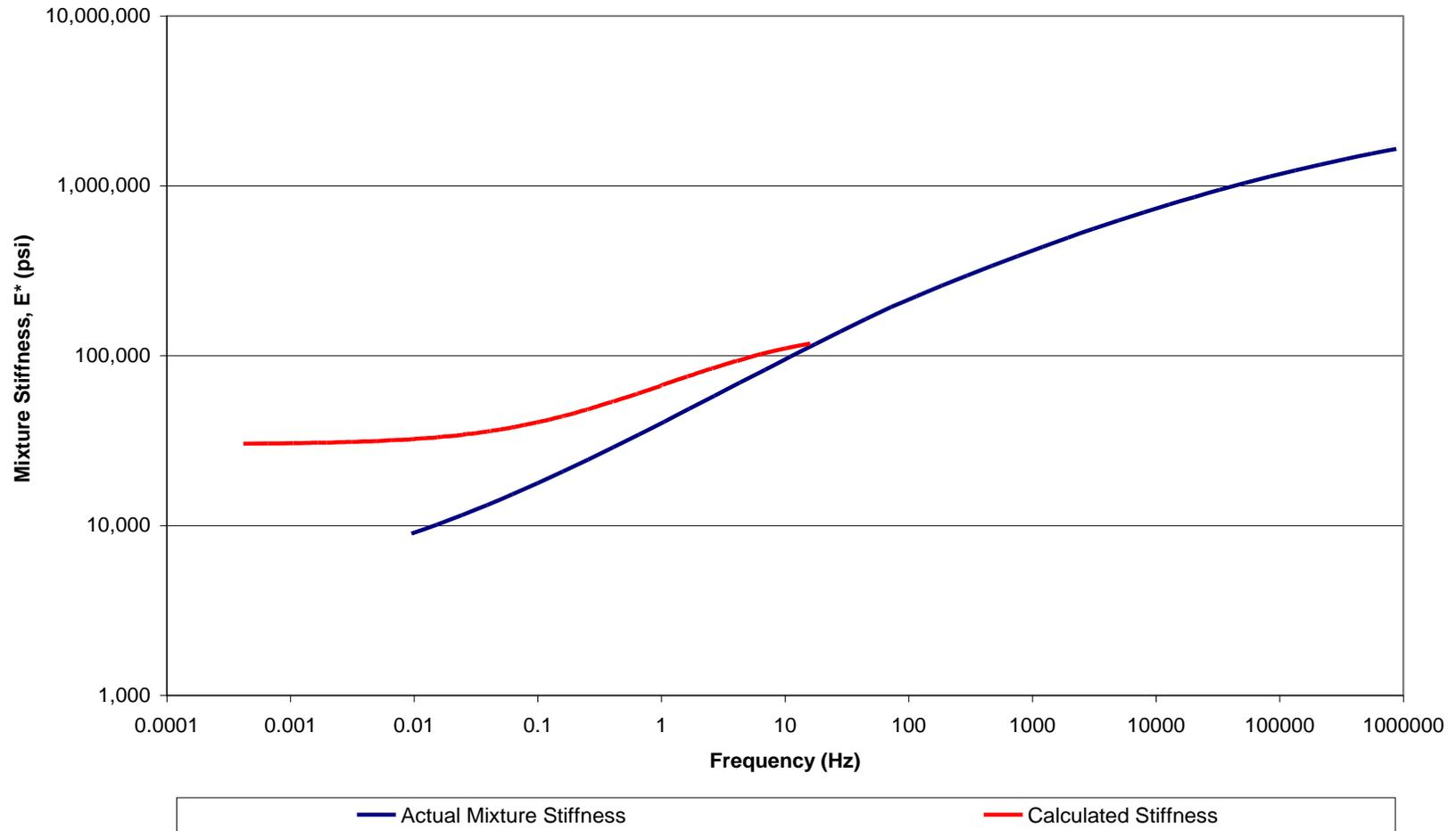
Figure 2: Measured and Predicted Stiffness Comparison ( $T_r = 40^\circ\text{C}$ )
