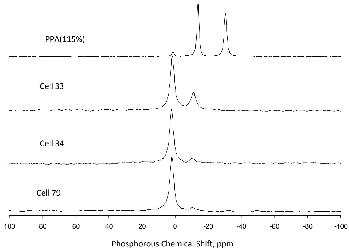
Figure 1.  $^{31}\text{P}$  NMR spectra of polyphosphoric acid (115%) and tank bitumens from MnROAD cells 33, 34, and 79.
