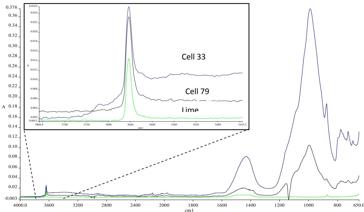
Figure 5. Infrared spectra of centrifuge fines extracted from cell 33 (blue) and cell 79 (black) and pure calcium hydroxide (green) showing the presence of lime in the centrifuge fines.
