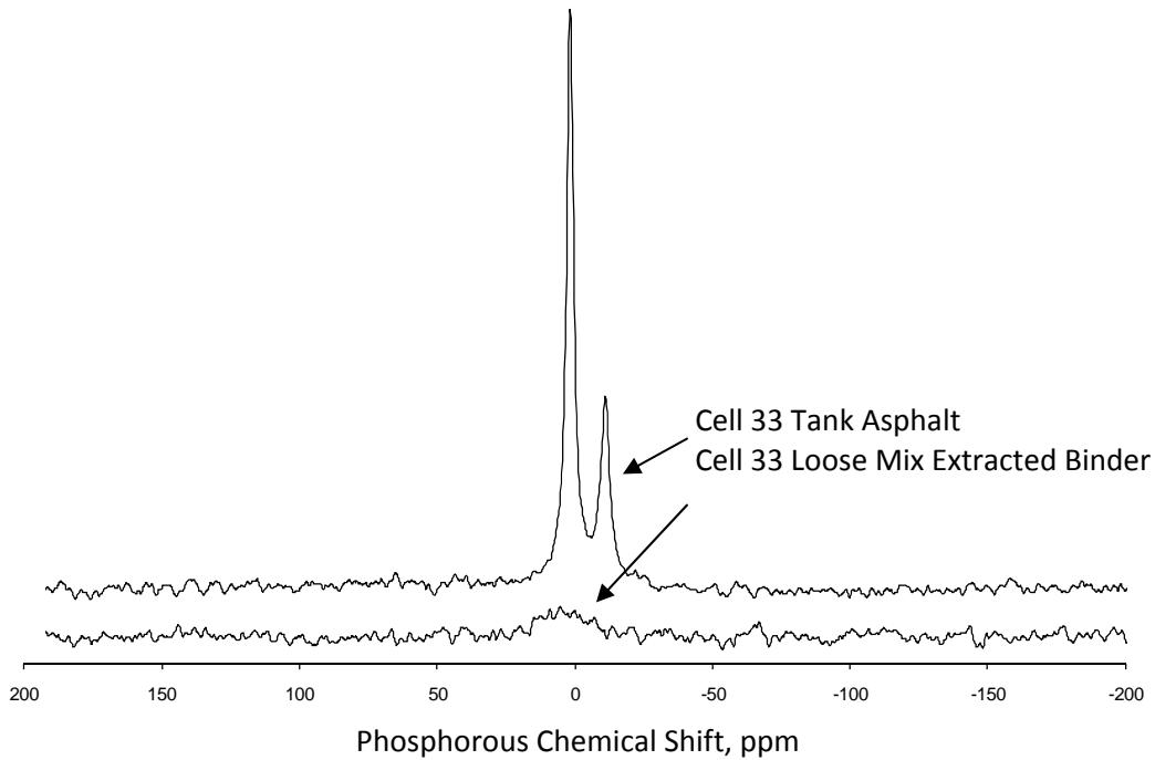
Figure 2. Liquid-state<sup>31</sup>P NMR spectra of MnRoad cell 33 tank bitumen and loose mix extracted binder illustrating the loss of soluble phosphorous NMR signal in the extracted binder .
