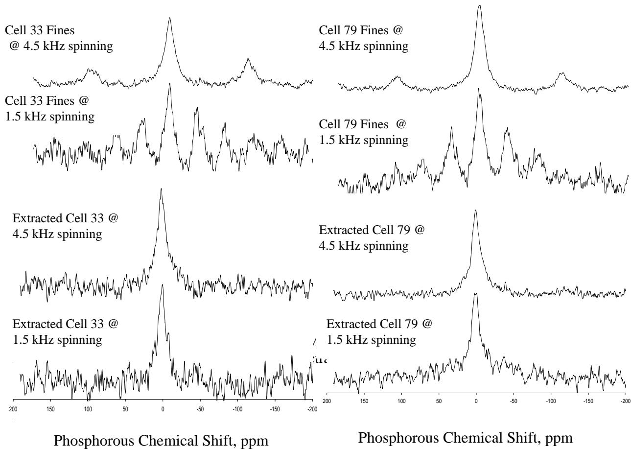
Figure 4 Solid-state Phosphorous NMR spectra of MN Road Cells 33 and 79 spinning at 1.5 and 4.5 kHz illustrating differences in the spinning sideband spectra between the fines and extracted binder.
