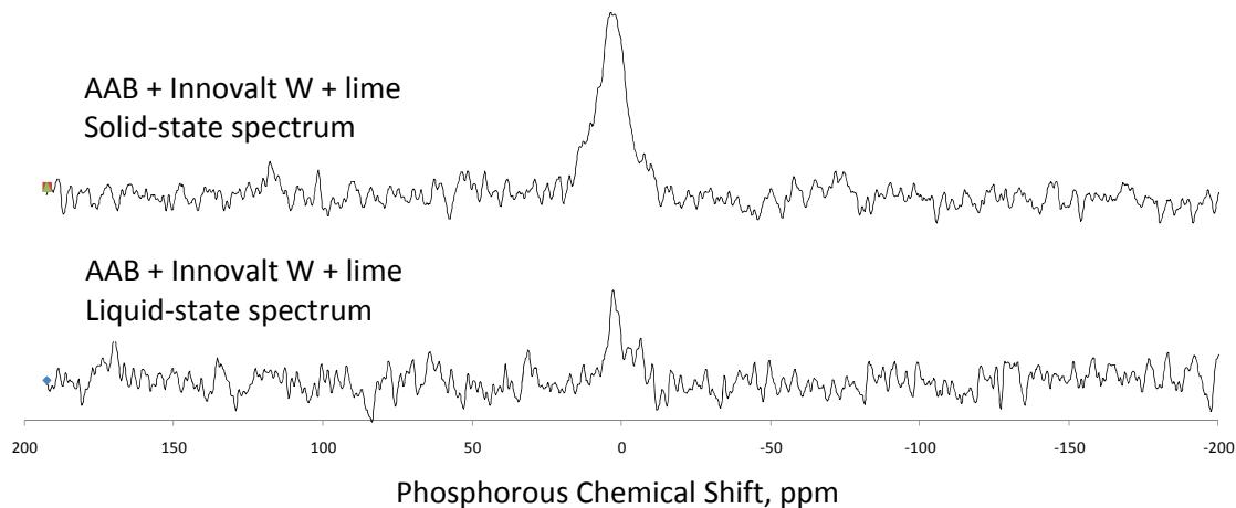
Figure 6.  $^{31}\text{P}$  NMR spectra of bitumen AAB-1, modified with 1% Innovolt-W and 5 % lime.
