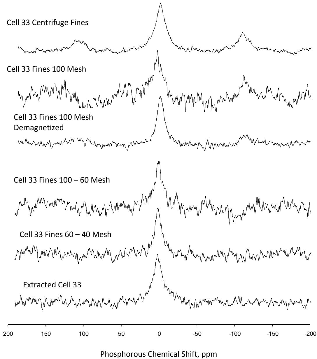
Figure 3 Solid-state  $^{31}\text{P}$  NMR spectra of fines from loose mix extracted binder in MnROAD cell 33.
