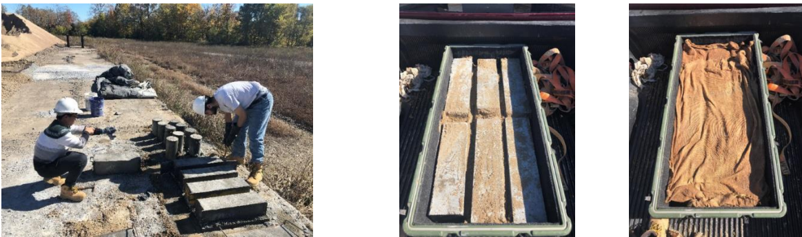
Figure 18 - demolding and transportation of samples
