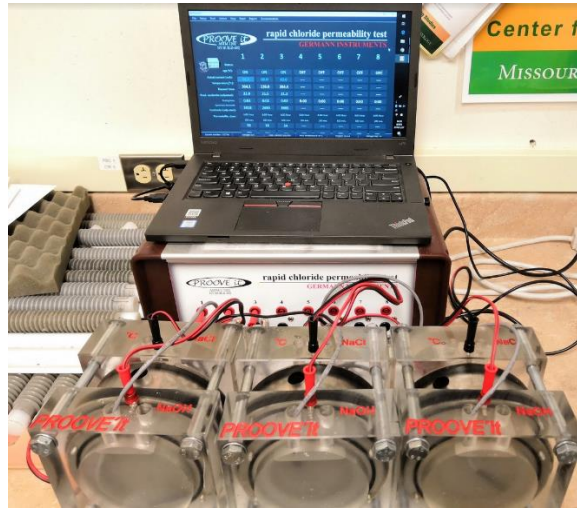
Figure 25 - Testing apparatus for RCPT
