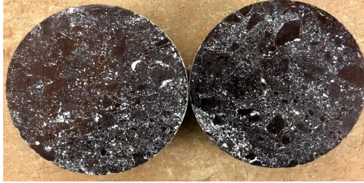
Figure 27 – Sample preparation for air-void system analysis
