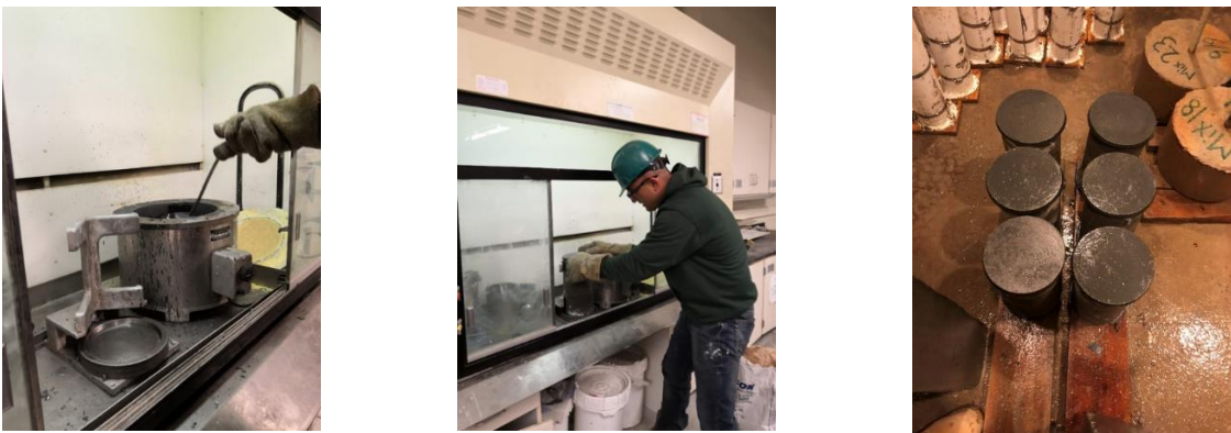
Figure 19 - Capping process of cylindrical samples
