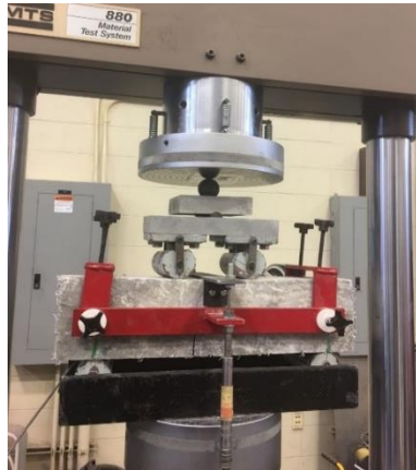
Figure 21 - Third-point flexural testing setup
