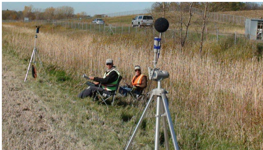
Figure 4.8. Statistical pass-by showing microphone and weather station near Cell 8.
