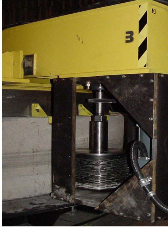
Figure 2.1. Grinding head developed by IGGA.
