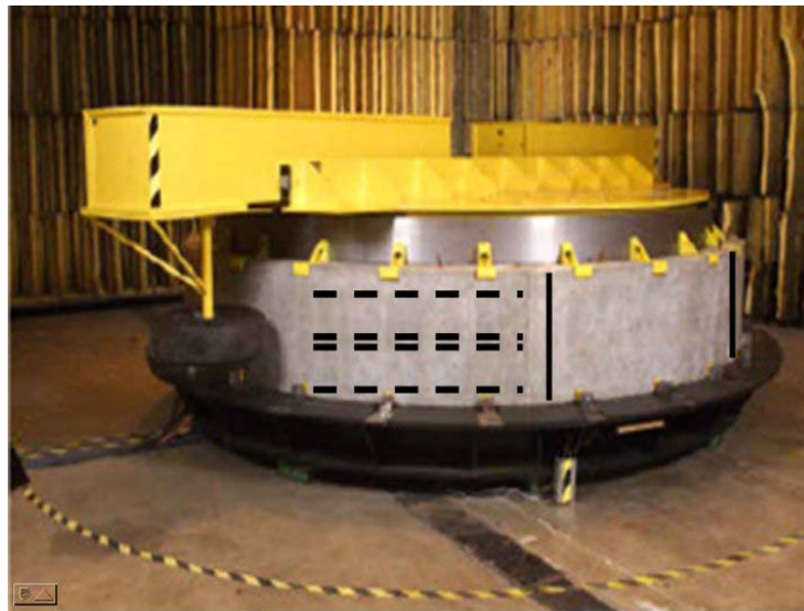
Figure 2.2. Top Track Purdue laboratory testing wheel and diamond grinder.
