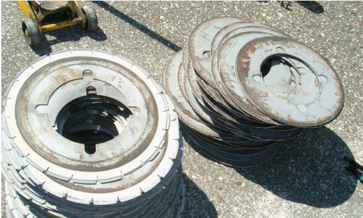
Figure 2.4. Grinding head and spacers.
