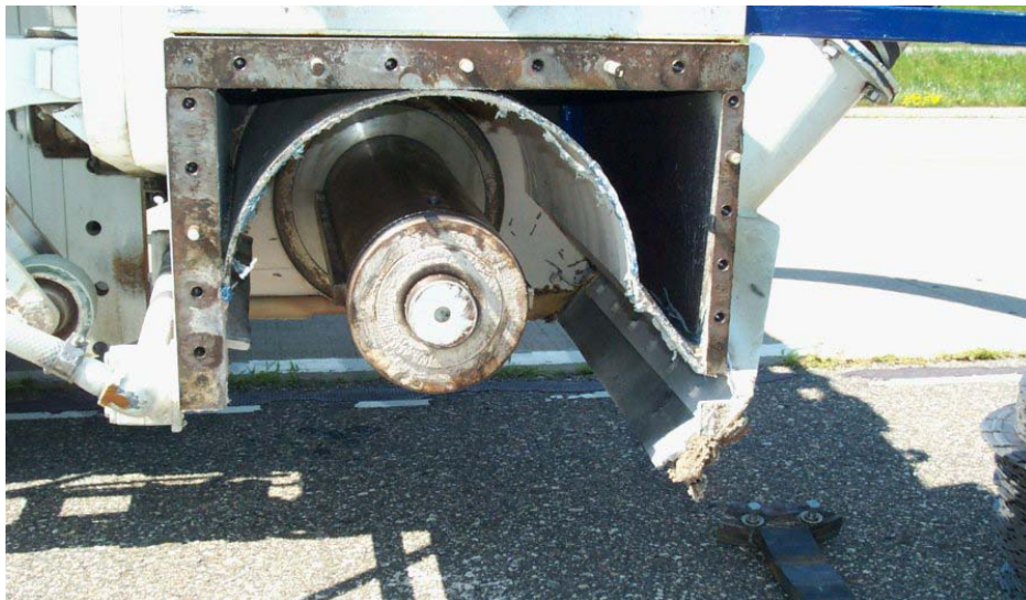
Figure 2.5. Grinding shaft before assemblage of cutters and spacers.
