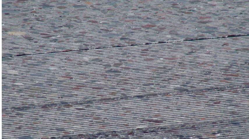
Figure 4.6. Innovative grind with skid marks after friction testing.
