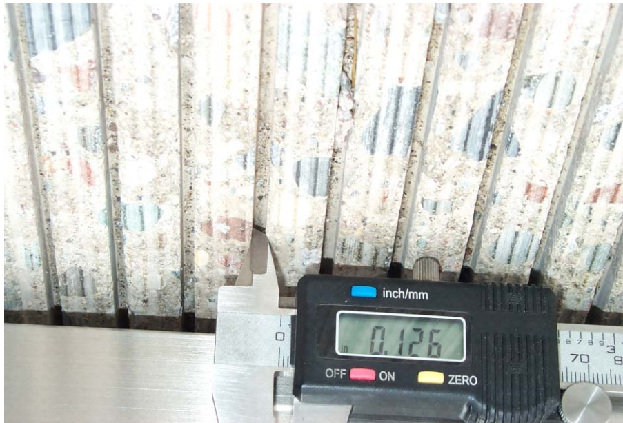
Figure 4.11. Ultimate grind groove width measurement.
