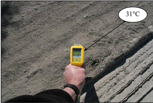
**Figure 7.28: Cement temperature prior to recycling (warm).**
