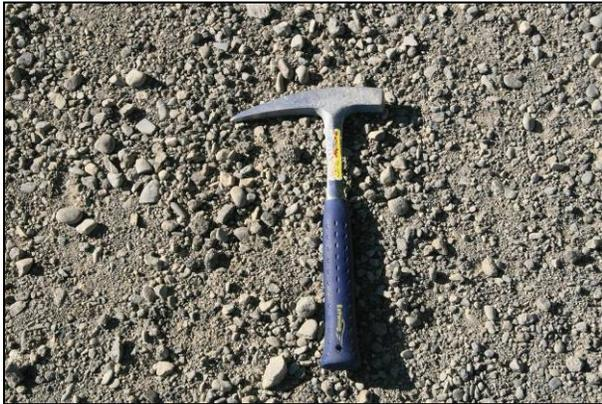
**Figure 7.34: Poor surface compaction in areas of recycling in cold temperatures.**
