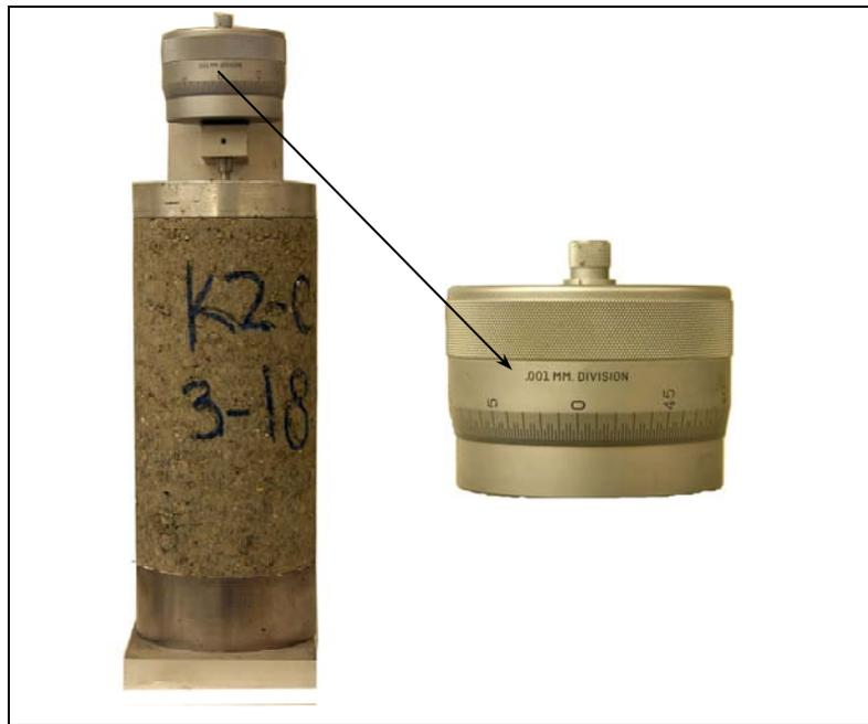
**Figure 9.17: Apparatus for measuring shrinkage of cured specimens.**
