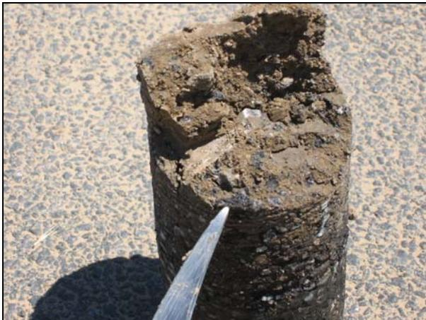
Figure 4.32: Core showing fines contamination. (2)
