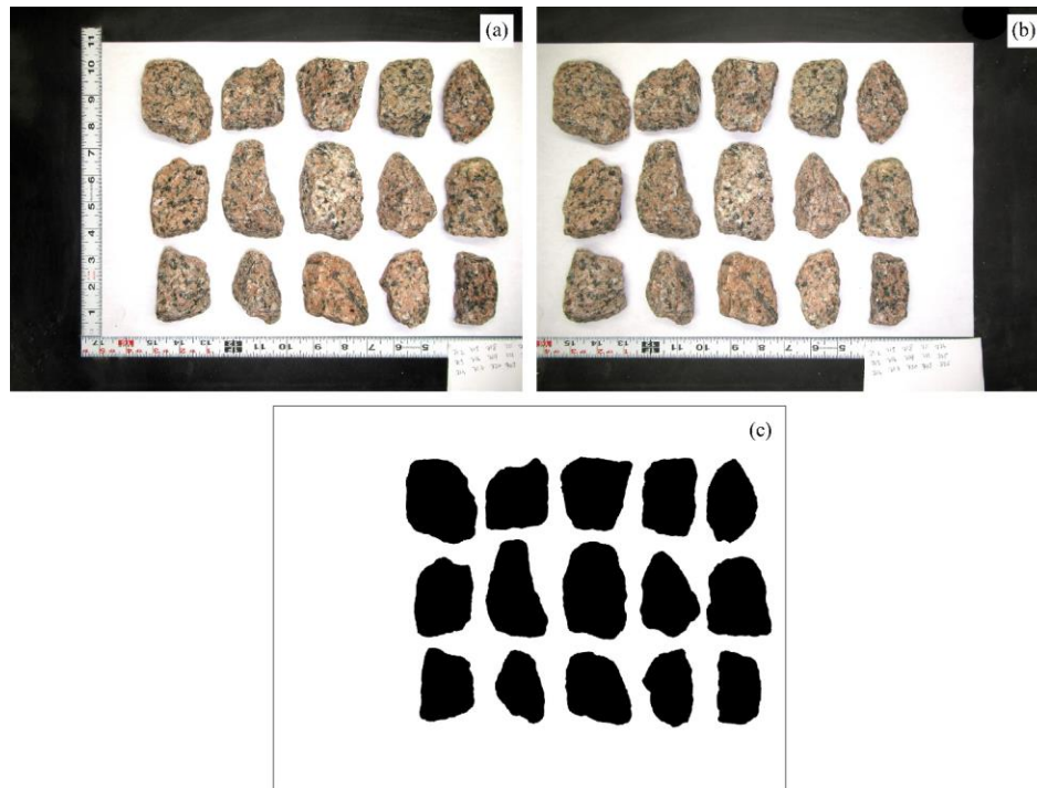
Figure 5.3. (a) Image taken from the left position, (b) image taken from the right position, and (c) binary image for LSSB material
