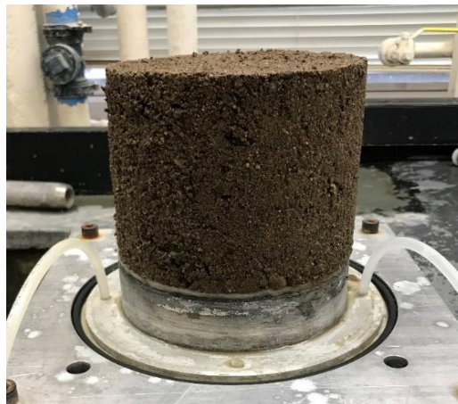
Figure 4.7. Specimen prepared in the compaction mold for the falling head permeability test
