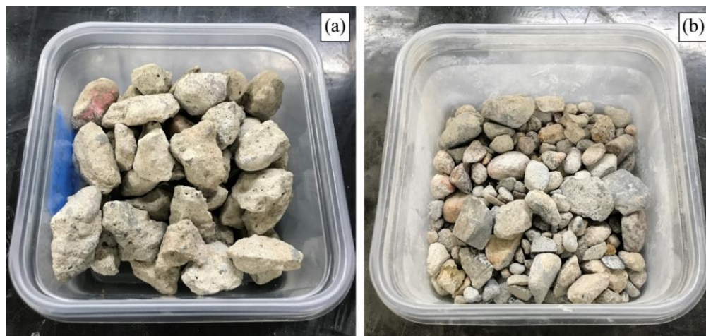
Figure 3.11. (a) Before the residual mortar content determination test and (b) after the test
