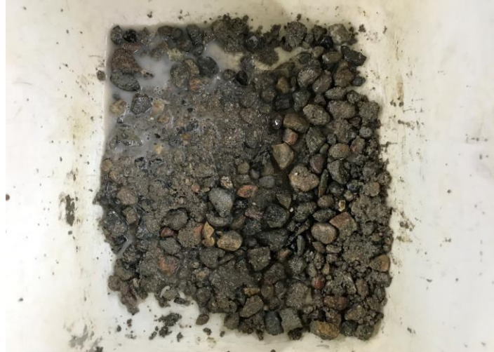
Figure 3.9. Mixture of the disintegrated mortar and aggregates
