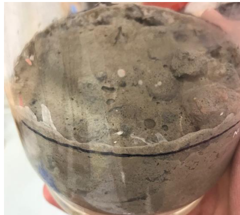
Figure 4.20. Cementation of Fine RCA after the hanging column test
