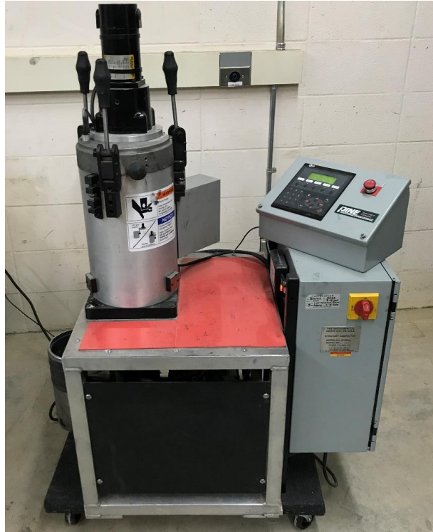
Figure 6.2. Picture of the gyratory compactor used in this study
