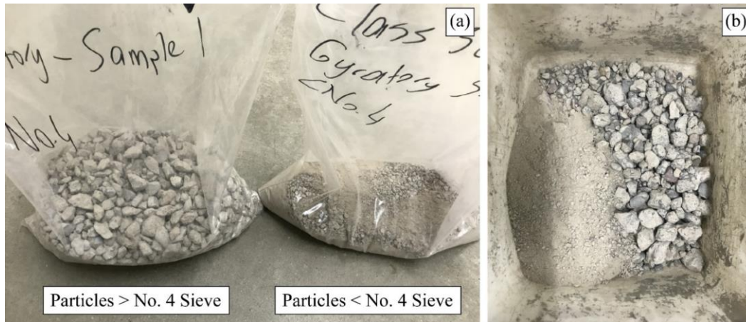
Figure 6.1. (a) Particle groups stored in different sealed bags and (b) mixing all particle groups prior to gyratory compaction
