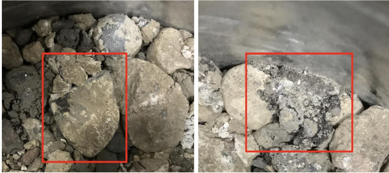
Figure 6.3. Examples of crushed particles after gyratory compaction
