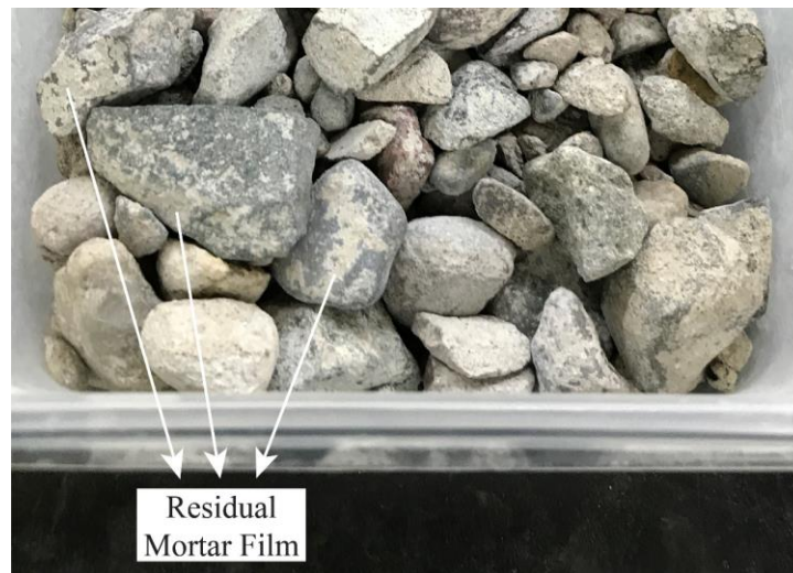
Figure 3.10. Remaining mortar film on the particle surfaces
