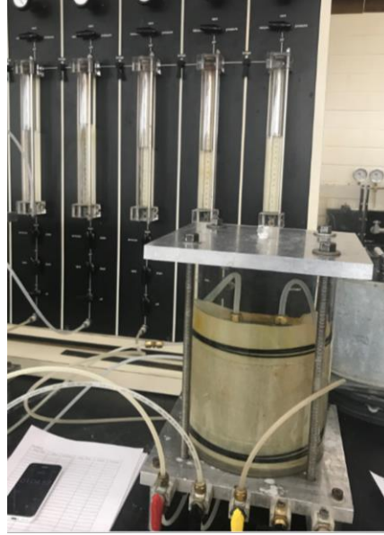
Figure 4.8. Picture of the falling head permeability test system
