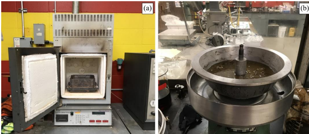
Figure 3.3. (a) Ignition furnace used in the ignition method and (b) asphalt extraction bowl used in the quantitative extraction
