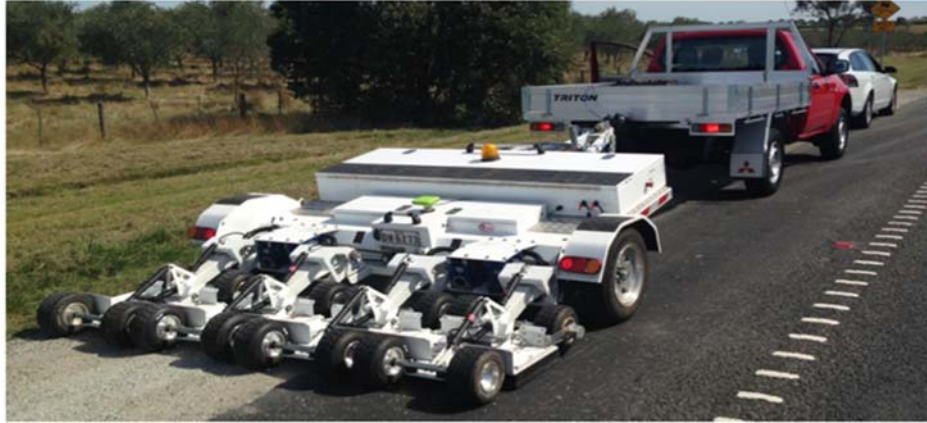
Figure 20. Second Generation NM-GPR System incorporating a Traffic-Speed 3D Ground-Coupled Antenna Array (Muller, 2017)
