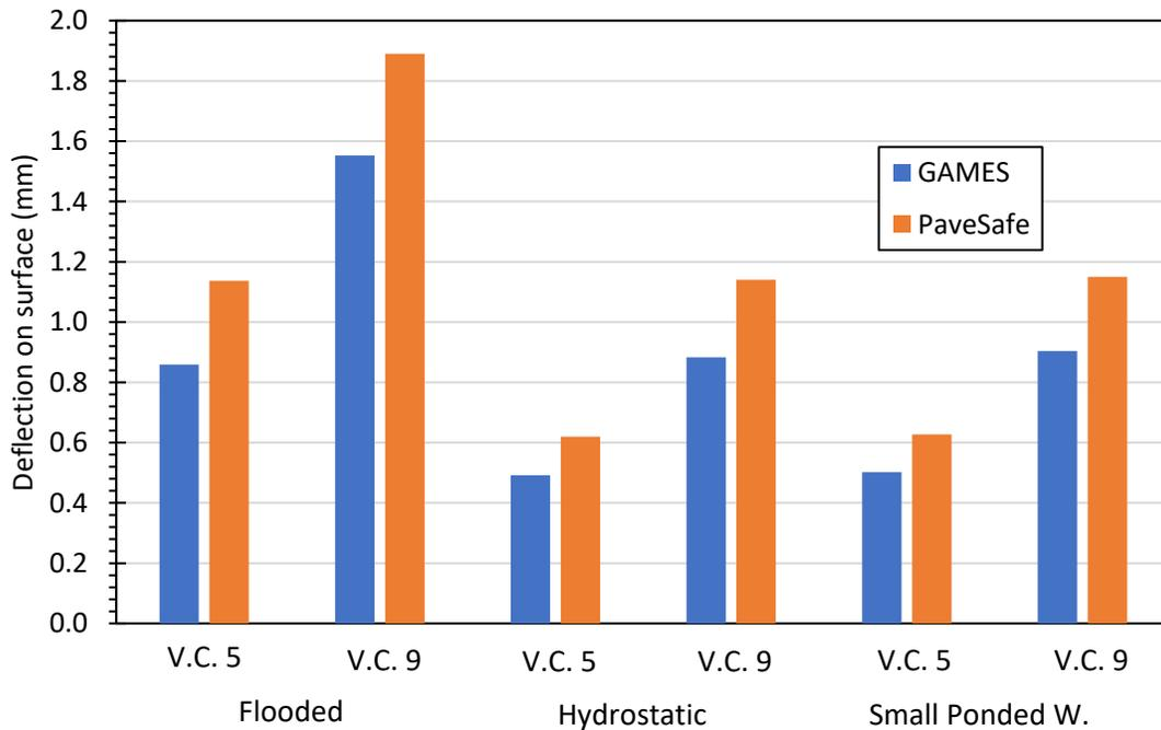
Figure 2-7. Comparison results from GAMES and PaveSafe for the three scenarios with A-7-6 subgrade type for vehicle class (V.C.) 5 and 9.
