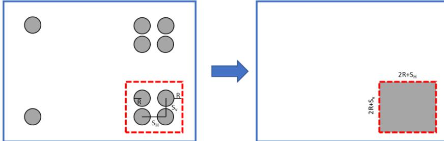
**Figure 2-5. Conceptual example of the equivalent footprint method for calculation of induced pressure and radius on AC surface.**
