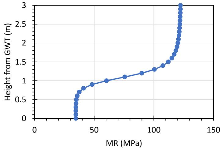
**Figure 2-3: Resilient Modulus profile for the hydrostatic scenario with AASHTO A-3 soil type.**
