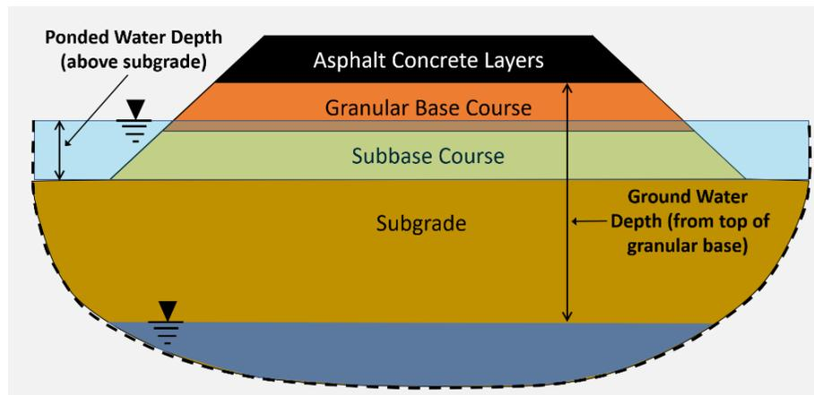
Figure 2-1. Schematic of the pavement cross section.
