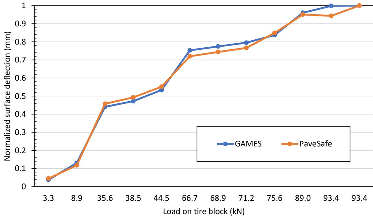
**Figure 2-9. Normalized surface deflection for all axle loads in hydrostatic scenario with A-3 subgrade type from GAMES and PaveSafe.**
