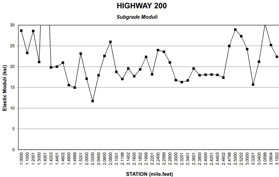
**Figure 3-1. Resilient Modulus of subgrade on ND 200.**
