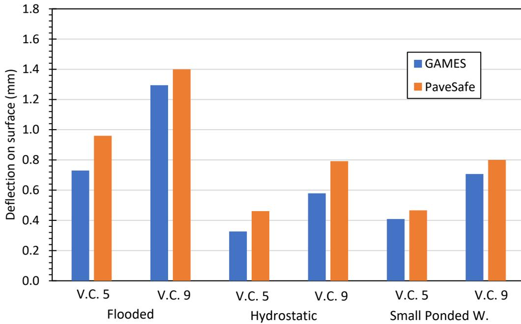
Figure 2-6. Comparison results from GAMES and PaveSafe for the three scenarios with A-3 subgrade type for vehicle class (V.C.) 5 and 9.
