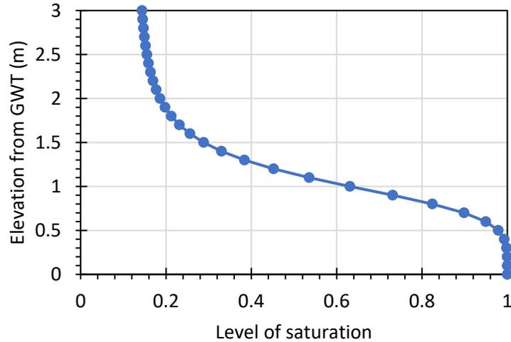
**Figure 2-2. Saturation profile for the hydrostatic scenario with AASHTO A-3 soil type.**
