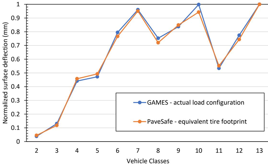
Figure 2-8. Normalized surface deflection for all vehicle classes in hydrostatic scenario with A-3 subgrade type from GAMES and PaveSafe.
