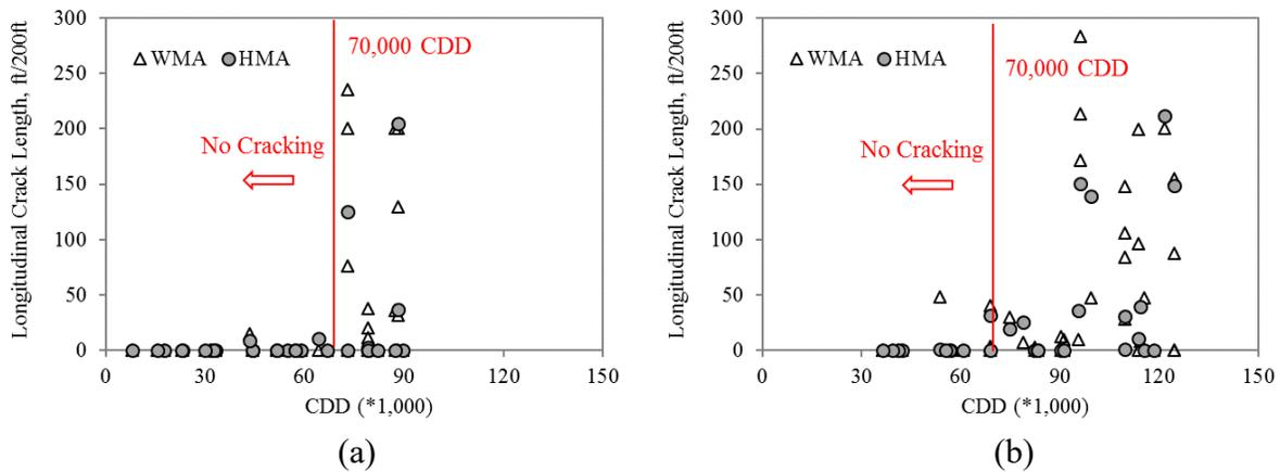
**FIGURE 1 Wheel-path Longitudinal Crack Survey Results; (a) First Survey in 2012/2013, (b) Second Survey in 2014/2015 (Shen et al., 2017)**
