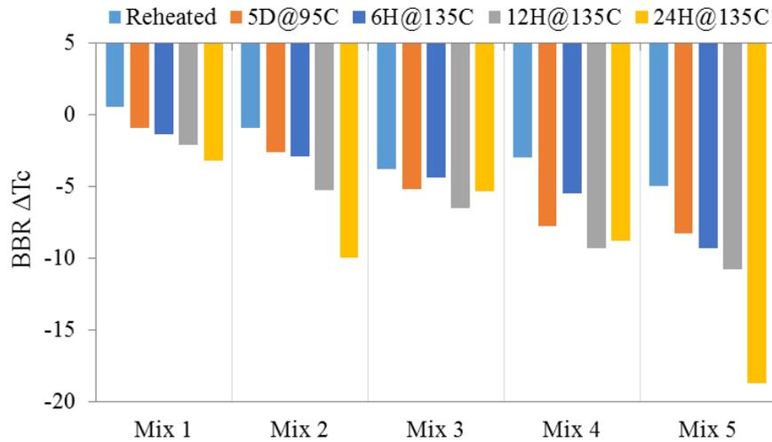
**FIGURE 6 BBR  $\Delta T_c$  Results of Extracted Asphalt Binders with Various Loose Mix Aging Protocols**
