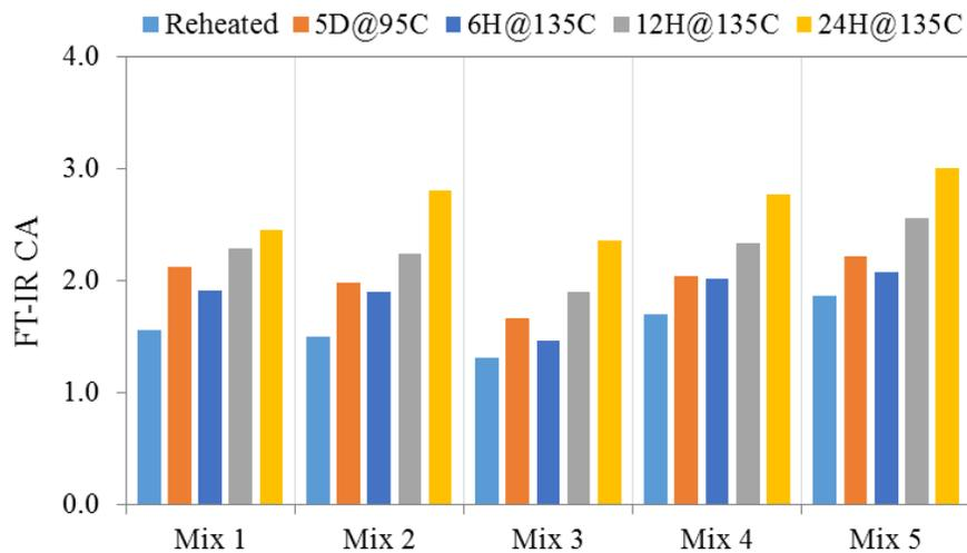
**FIGURE 7 FT-IR *CA* Results of Extracted Asphalt Binders with Various Loose Mix Aging Protocols**
