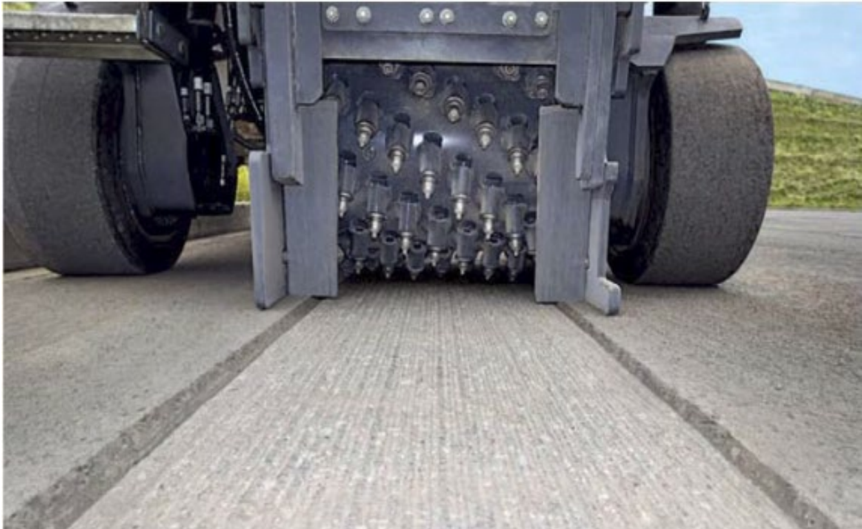
Figure 2.7 Staggered teeth on the milling (Wirtgen, 2018).
