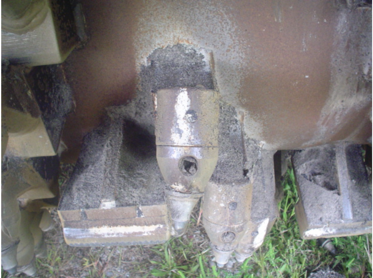
Figure 2.3 Misaligned tool on tooth holder (Baker, 2014)
