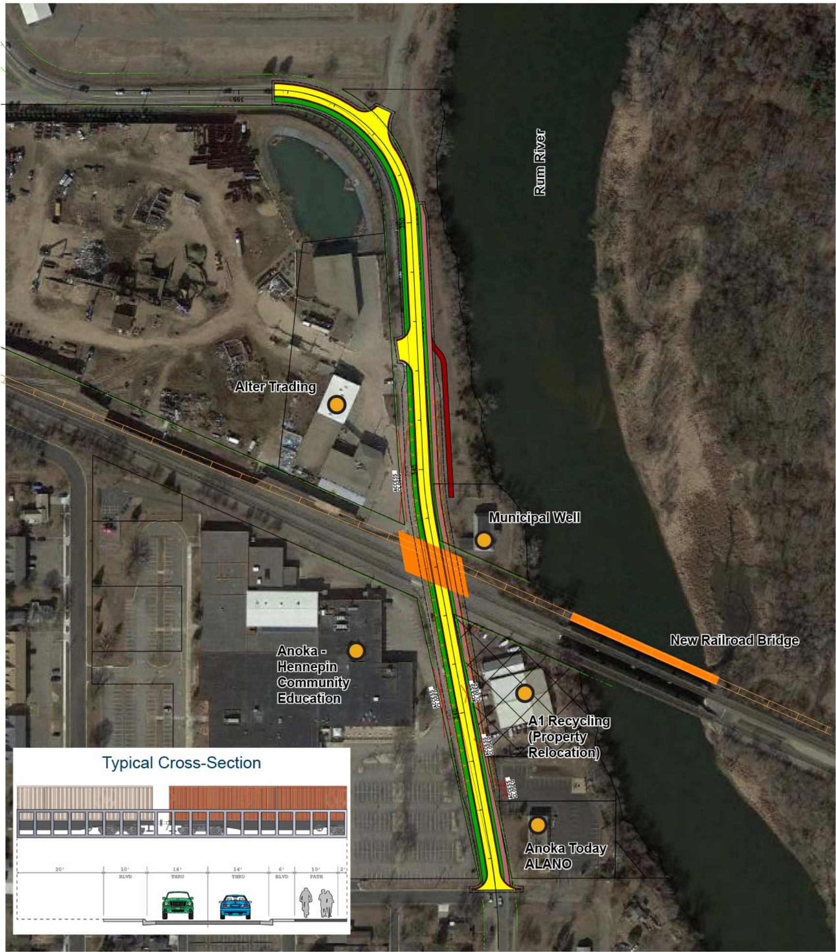
Figure 3: Concept for Alternative with Road Under the Railroad
