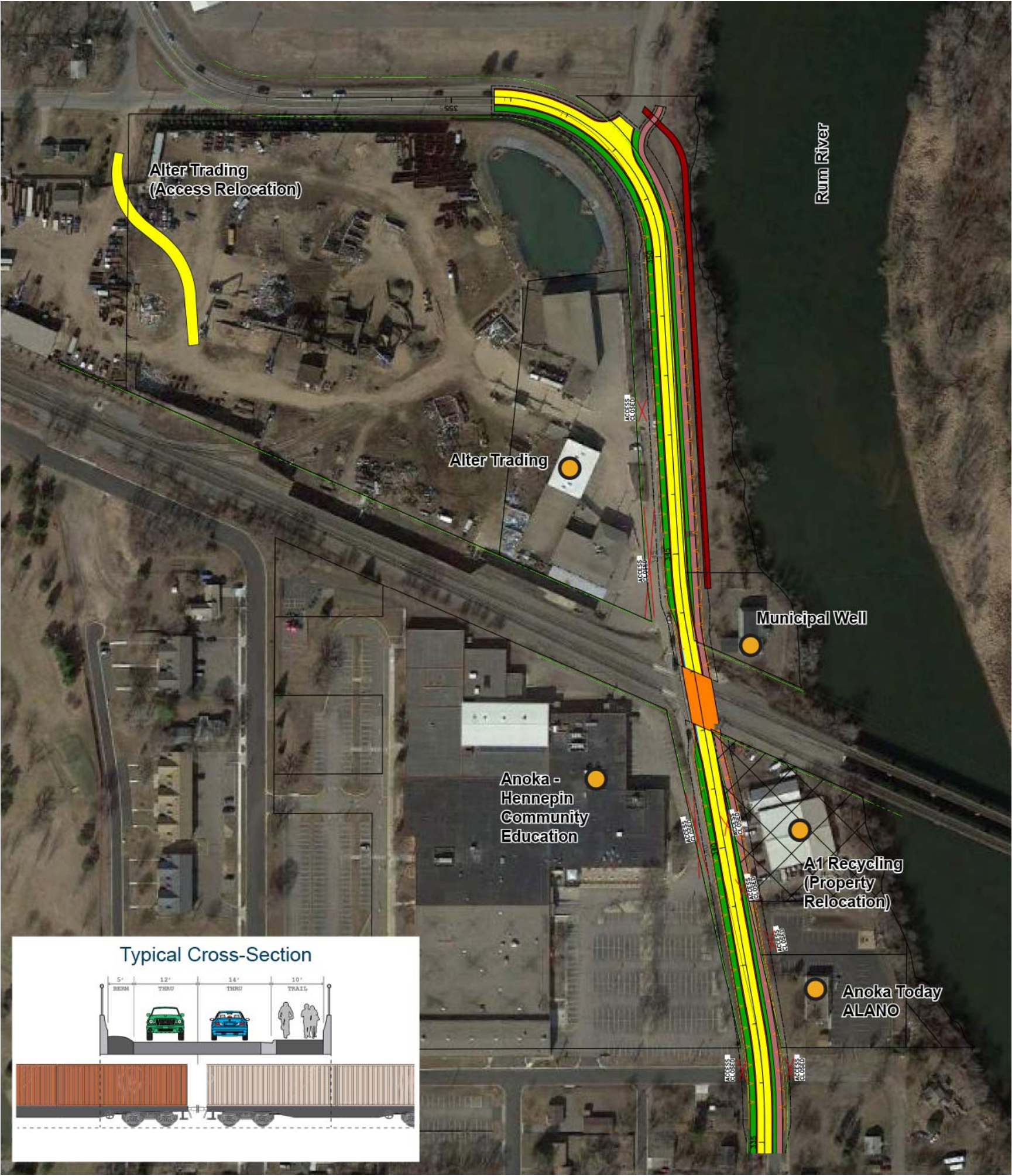
Figure 2: Concept for Alternative with Road Over the Railroad
