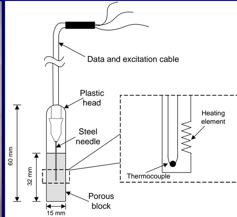
Schematic of Thermal Dissipation Sensor – Model 229 by Campbell Scientific Inc.
