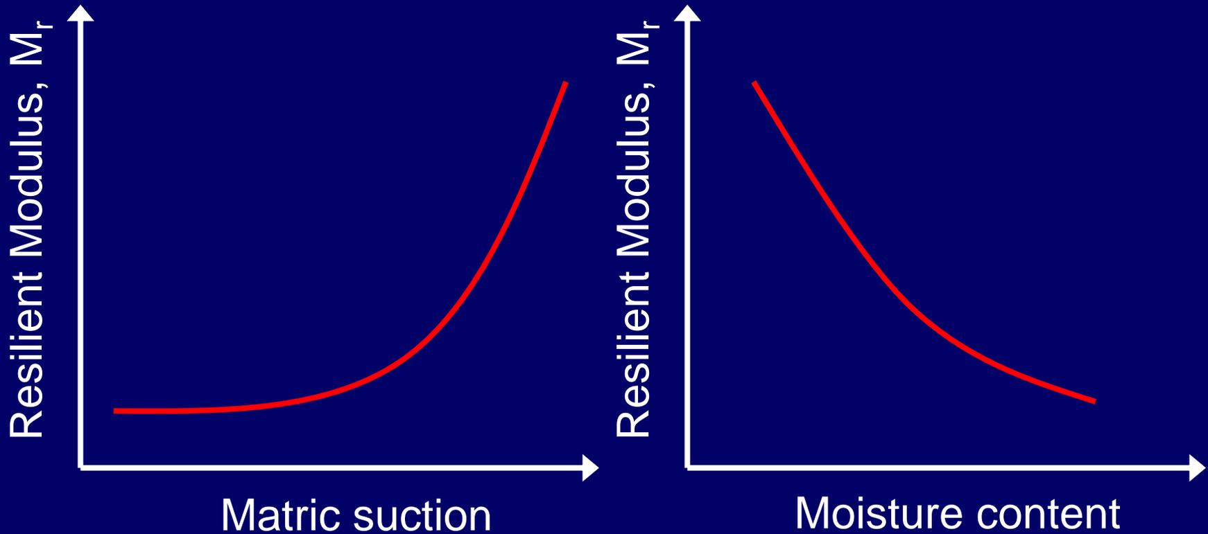
Modulus of unsaturated soils is strongly influenced by matric suction, particularly for compacted fine-grained soils. However, simple predictive relationships between  $M_r$  and matric suction have not been defined.
