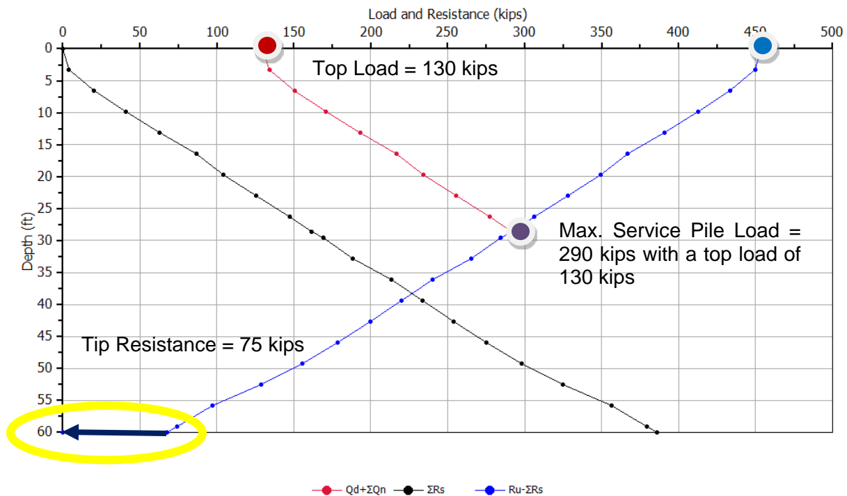
Figure F-7-6: The 60 foot deep pile is modeled here with a 50% mobilized tip capacity (75 kips). This reduced contribution of tip resistance is likely a more realistic loading at the service limit where loads are well below the strength limit (and correspondingly mobilized resistances are less than the maximum used for Strength Limit calculations).
