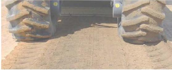
Minimal material sticking to the wheels of the recycler
