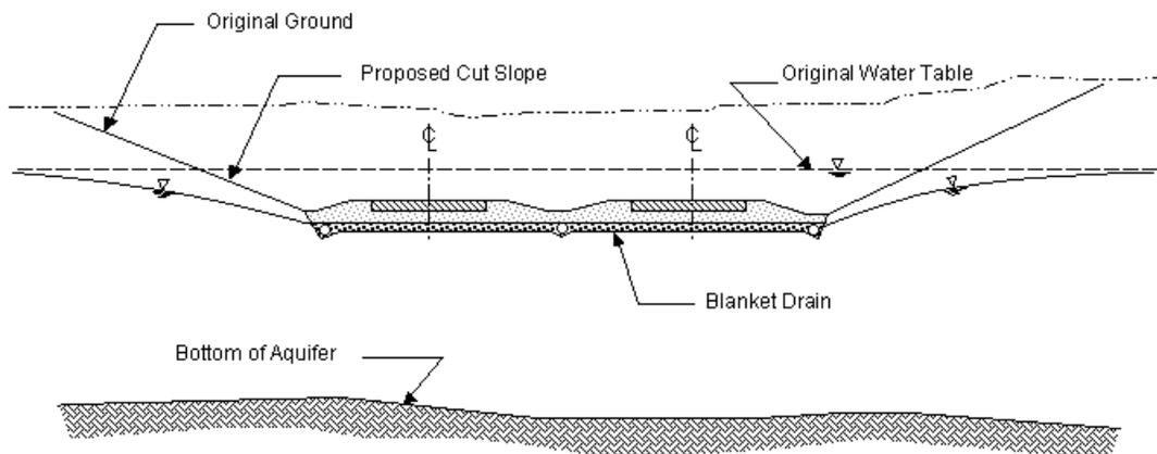
These two drainage systems may also be used together on a particular project. This is common on high profile projects where failure of one system could cause closure of a multilane highway and effect many people. The redundancy of two systems would lessen the chance of that occurring.
