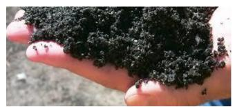
Figure 200.13 – Recycled Asphalt Shingles
