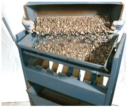
Figure 700.1 - Riffle Splitter
