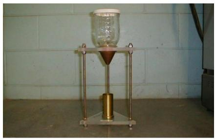
Figure 700.7 – FAA Apparatus
