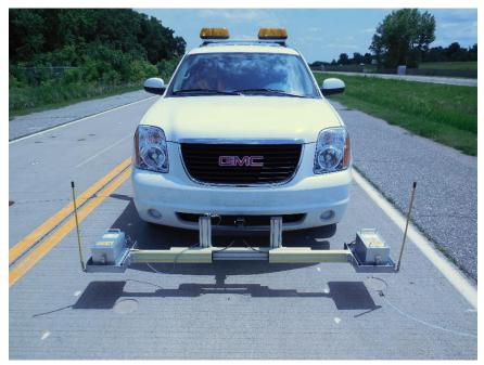
Figure 500.29 – Inertial Profiler
