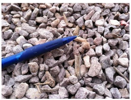
**Figure 200.18** – Aggregate mix contaminated with pieces of wood, which is considered deleterious material.
