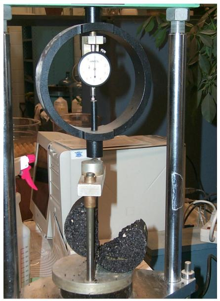
Figure 300.3 – Apparatus used to perform a Lottman test.
