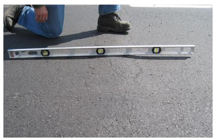
Figure 600.28 – Bump over concrete joint
