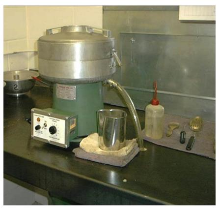
Figure 700.6 – Centrifuge Extractor
