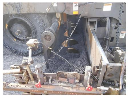
**Figure 600.19** – This photo shows the correct material head in front of the screed. However, auger extensions should have been used in this case.
