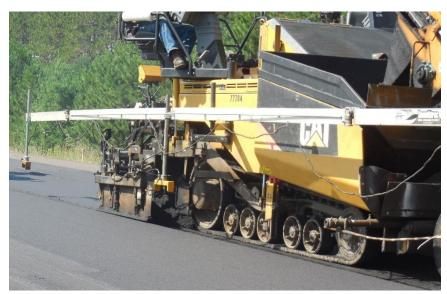
Figure 500.16 – A tracked paver using sonic sensors to adjust the screed.
