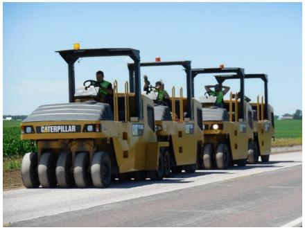
Figure 500.19 – Pneumatic Tired Rollers.
