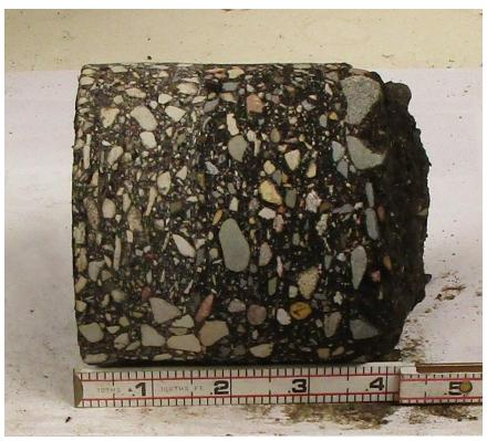
**Figure 100.20** – Stripping of an asphalt core from the bottom of the asphalt layer.
