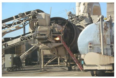
Figure 400.4 – Parallel-Flow Mixing Drum
