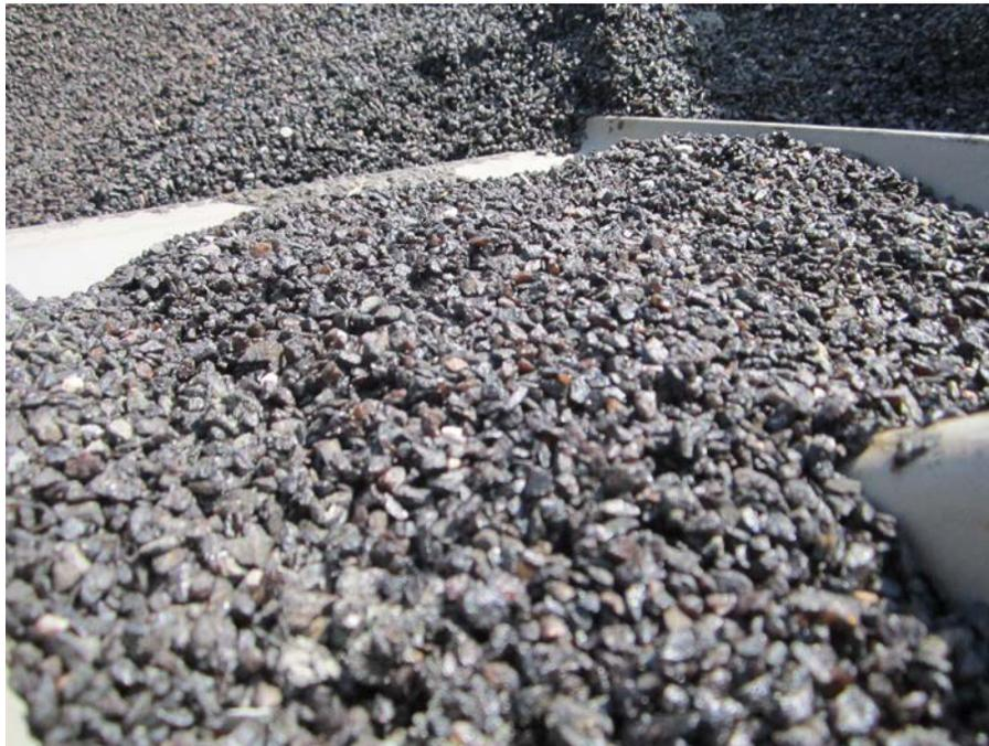
**Figure 2 – Pre-coated stone used for entire project**
