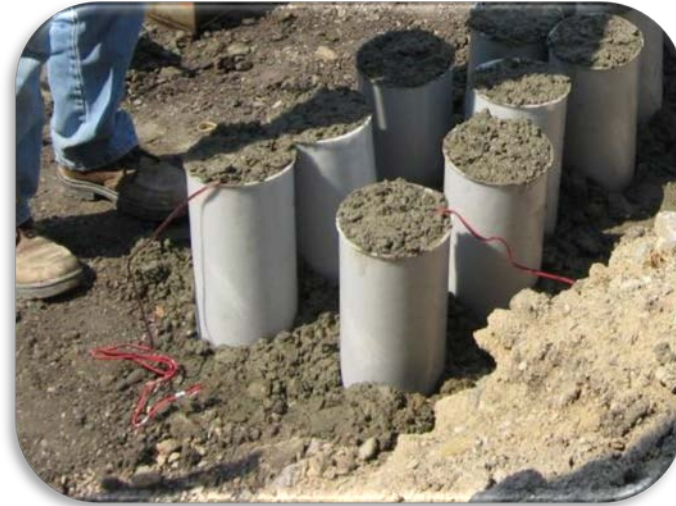
Embed the sensors in the center of the 2 additional beams or cylinders specimens
