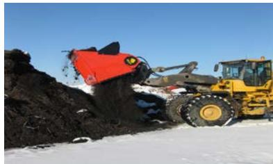
The ALLU screener buckets have been developed for larger processing jobs. Everything from aerating compost, primary on-site screening and processing construction material.
