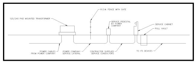
Most power companies no longer allow MnDOT equipment on their power poles and many are using service pedestals. It is important to note that most power companies prefer the meter to be less than 15 feet from the service pedestal or pad mounted transformer.
