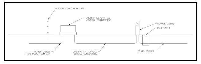
*Figure 3-5: Typical Power Service - Ground-Mounted Transformer outside MnDOT R.O.W. with Service Pedestal within MnDOT R.O.W.*
