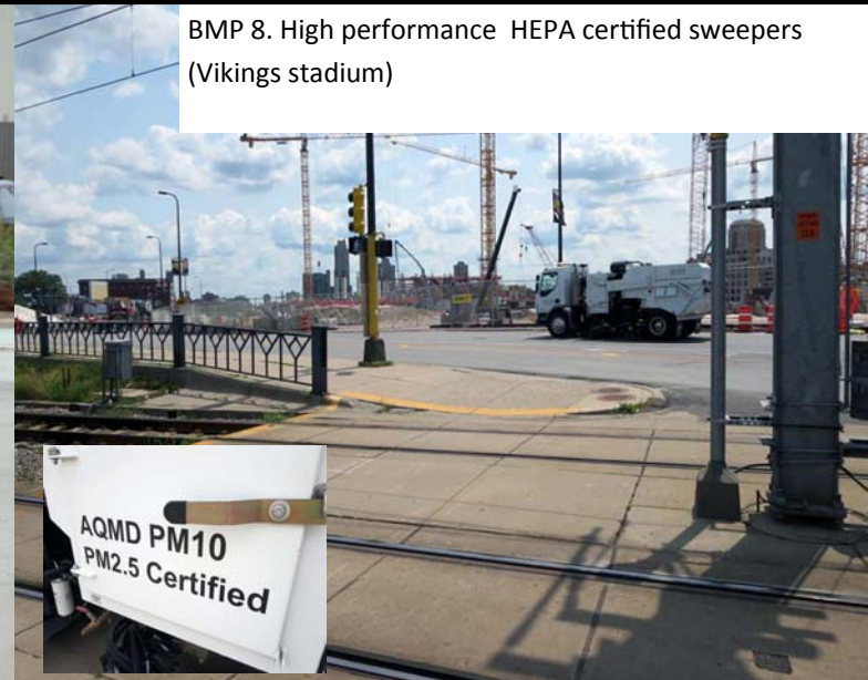
BMP 8. HEPA filter sweeper attachment to pickup broom
