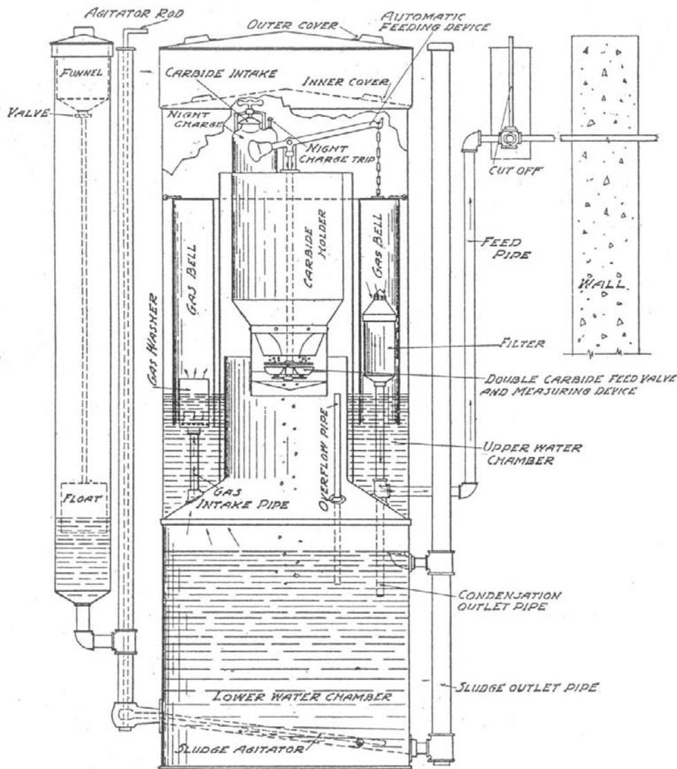
This acetylene or carbide gas plant was designed to be buried in a pit about 12' deep. The pit was usually located 50' to 100' from the farmhouse. Ground-level evidence of such a pit might include a circular pit cover, an agitator rod, and pipes, all located within an 8'-diameter circle. From Mowry's *Lighting Farm Buildings* (1915).
