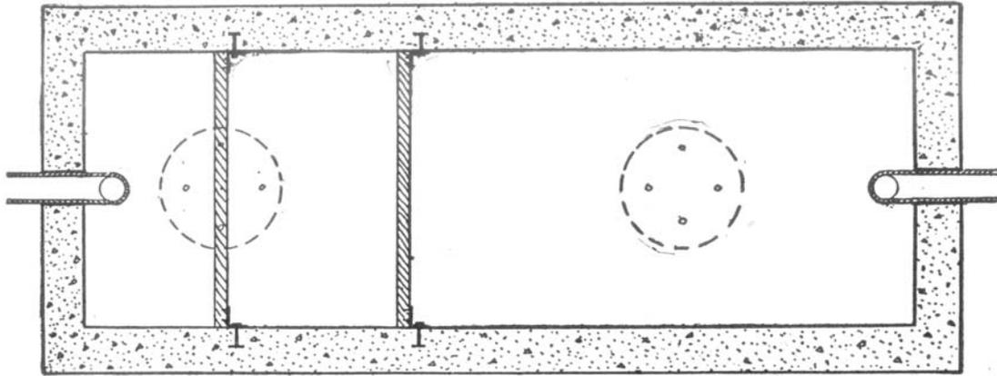
Fig. 35.—Top View of Septic Tank.
