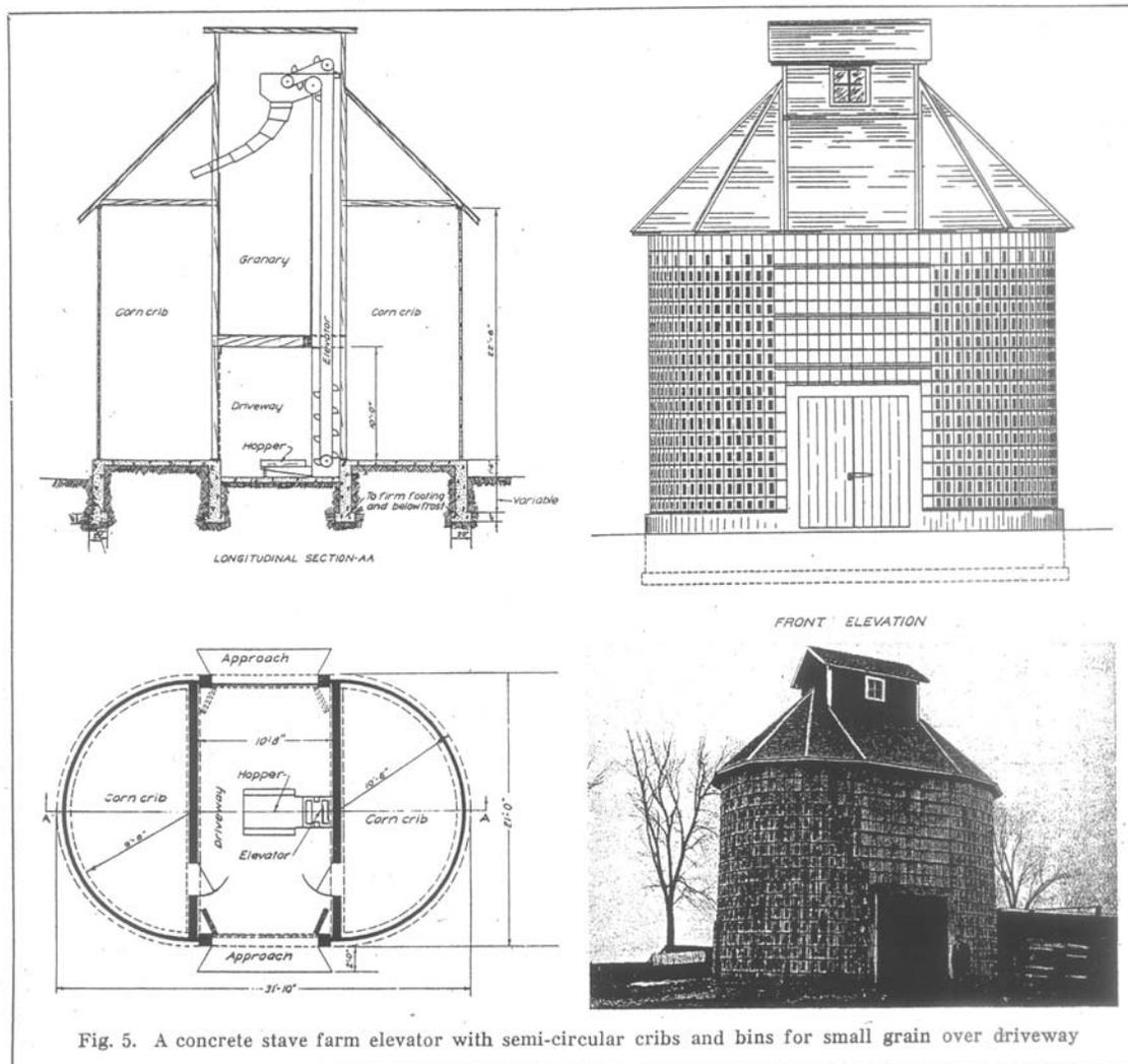
Fig. 5. A concrete stave farm elevator with semi-circular cribs and bins for small grain over driveway
