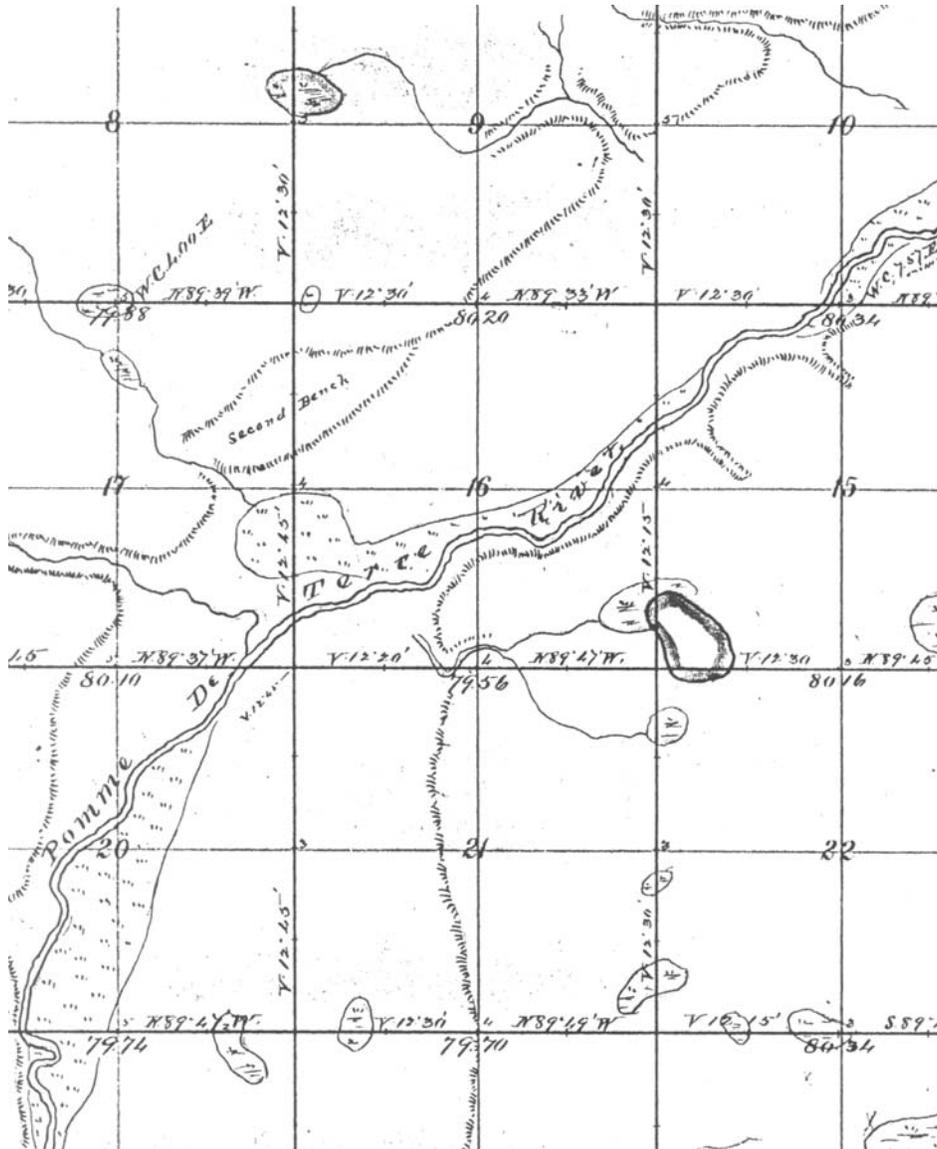
This map, dating from 1891, is an early copy of the surveyor's data that translated the township and range system of land division into real space. The original surveyors placed boundary markers or monuments on the land to mark the section and quarter-section lines. Maps like this are still used at county recorders' offices to form the basis for land ownership documentation. (Courtesy Stevens County Recorder's Office)
