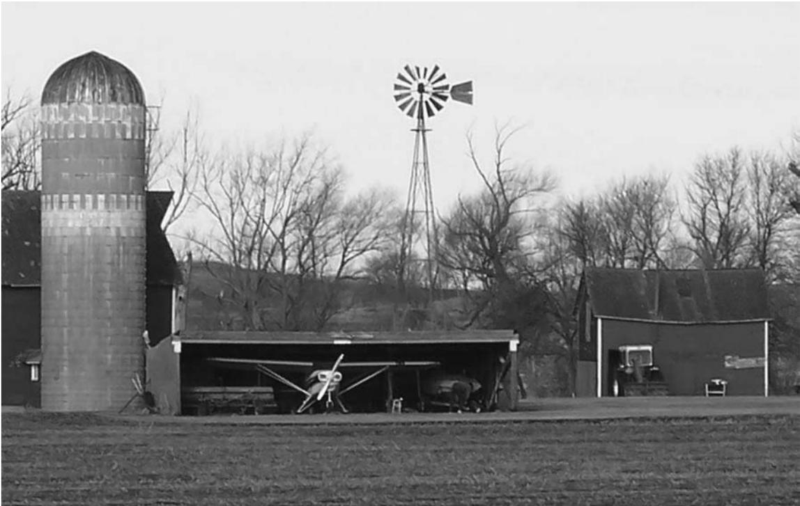
A typical western Minnesota farm hangar, sided with metal. Its eastern side is entirely open. The landing strip, still in use, is aligned north and south and is located along the edge of the field shown in the foreground. Solvie Farm, Pope County, 2005. (Gemini Research photo)
