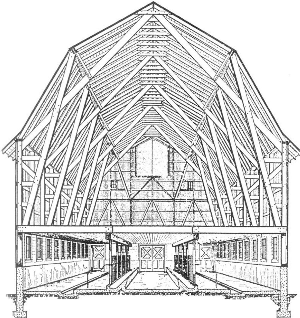
This 1946 illustration of a Shawver truss plank-frame barn appears in a recent essay by Glenn A. Harper and Steve Gordon on the 20th century development of Midwestern barns. According to the authors, "In the 'modern' plank-frame barn, roofs were supported by purlins which, in turn, were supported on specially designed, self-supporting trusses, or the roofs themselves were self-supporting" (1995: 217).
