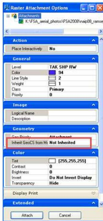
Another option in Raster Manager is to display the column “Inherit GeoCS from Model”. Right click on the column headings to display the popup menu and select the heading. Then click the checkmark off.
