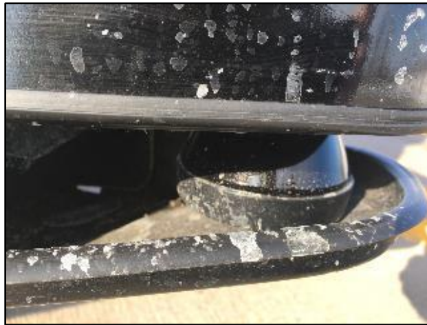
Figure 3-15 Road Salt on LIDAR Sensor
