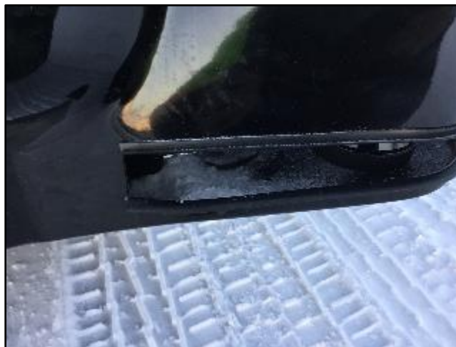
Figure 3-16 Snow Accumulation in Sensor Housing
