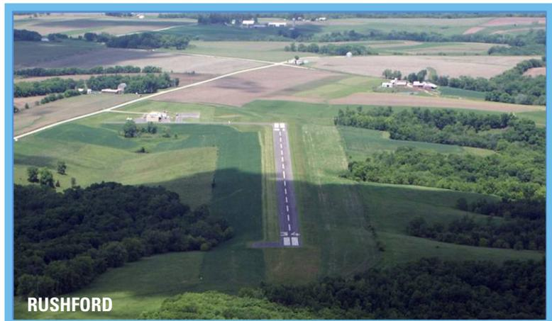
**Landing Strips:** Landing Strips have one or more turf runways which can accommodate most single-engine aircraft and some twin-engine aircraft. This type of airport may be unusable during certain conditions such as wet weather, winter months, and during the spring melt. A key function of these airports is supporting the agricultural industry with crop seeding and spraying services. There are currently 22 Landing Strip Airports in the state’s system.
