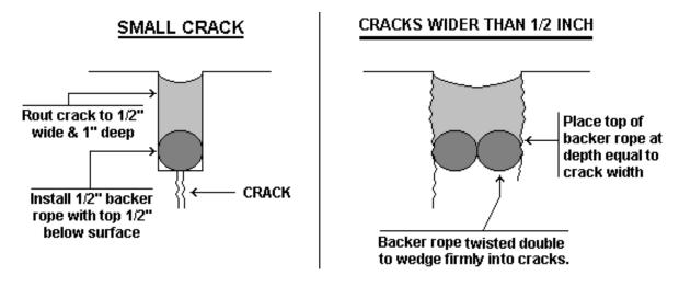
Figure 2. Crack sealing.
