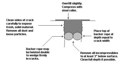
Figure 3. Overband sealing.
