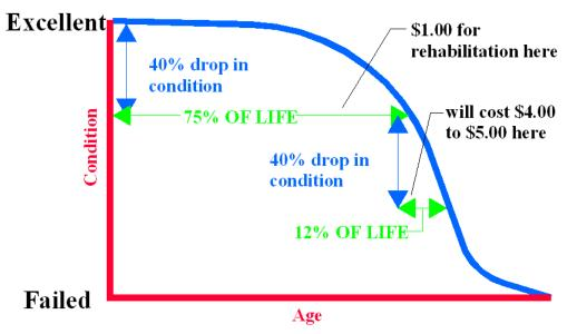
Figure 1. Pavement condition life cycle.
