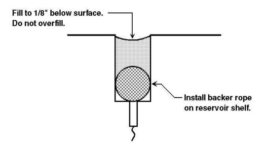
Figure 6. PCC joint/crack repair.
