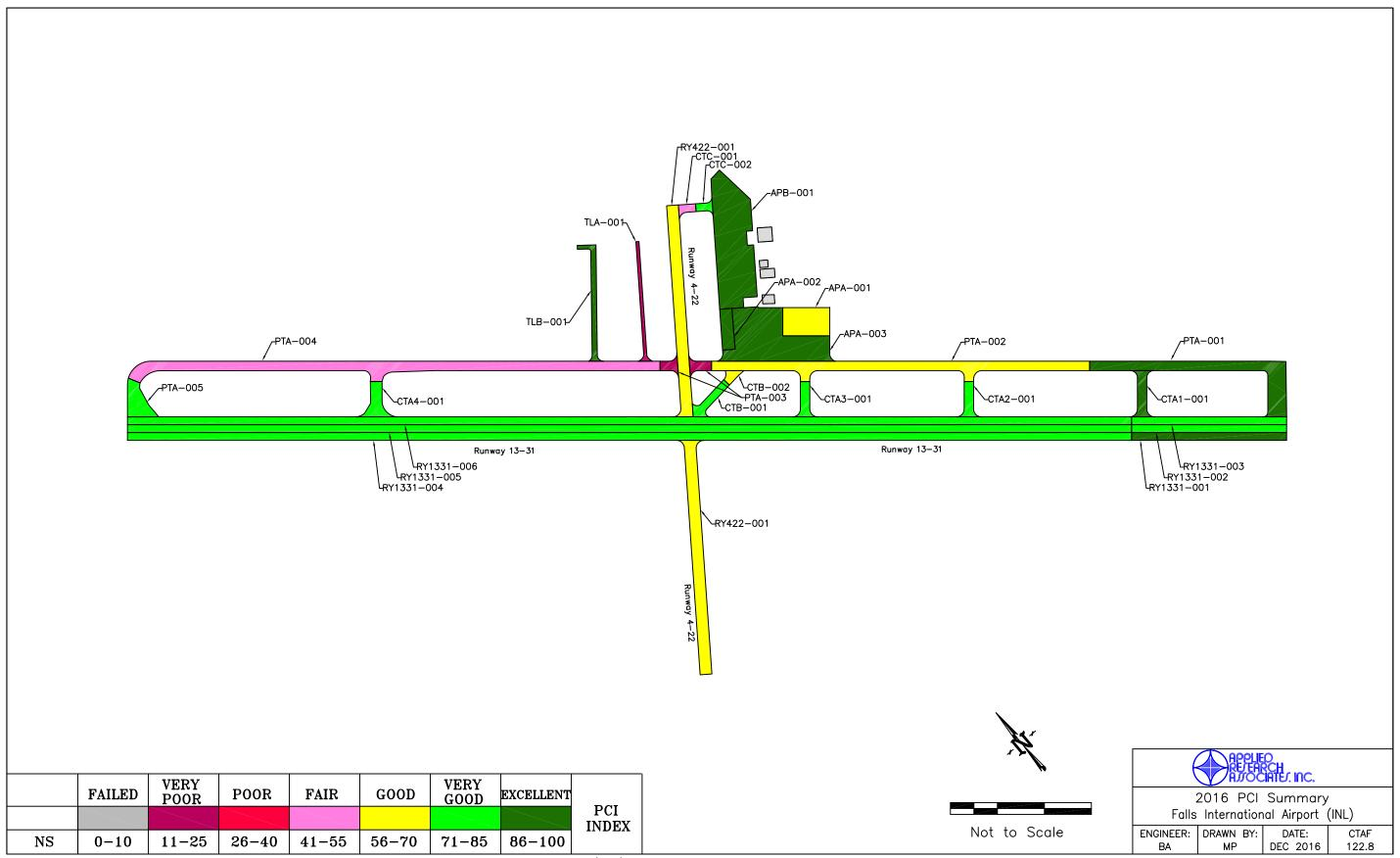
Figure 4. 2016 Pavement Condition Index Rating at Falls International Airport (INL).
