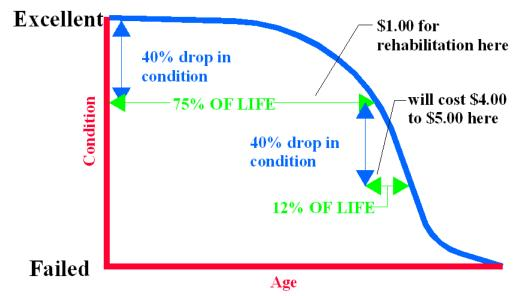
Figure 1. Pavement condition life cycle.
