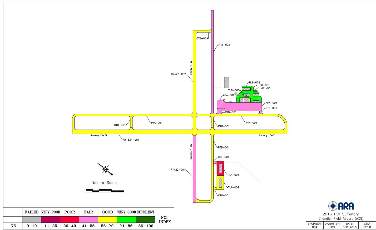
Figure 4. 2016 Pavement Condition Index Rating at Chandler Field Airport (AXN).
