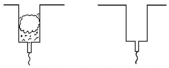
Typical joint with deficient sealant and a collection of debris & incompressibles.
