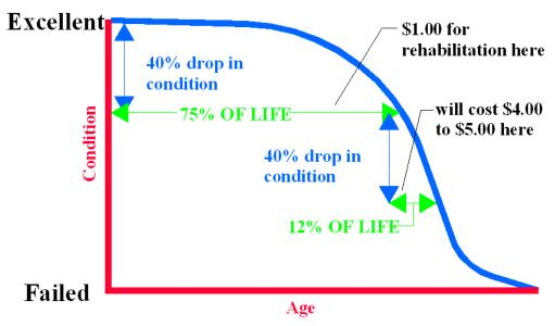
Figure 1. Pavement condition life cycle.
