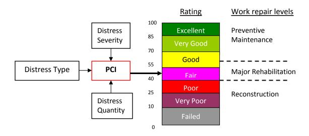
Figure 3. PCI rating scale and repair levels.
