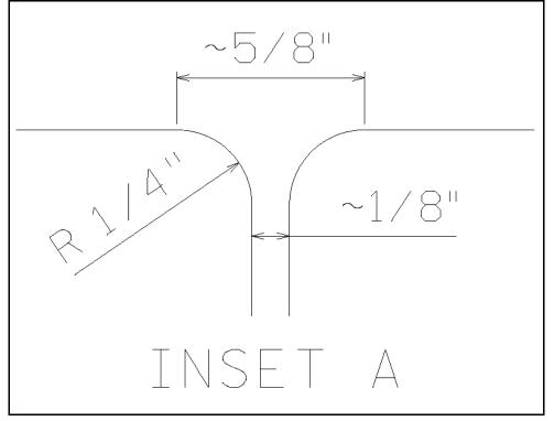
Figure 10b - Spec 2521.3c (allowable joint displacement)
