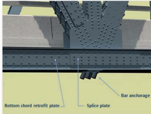
Proposed typical through truss bottom chord connection
