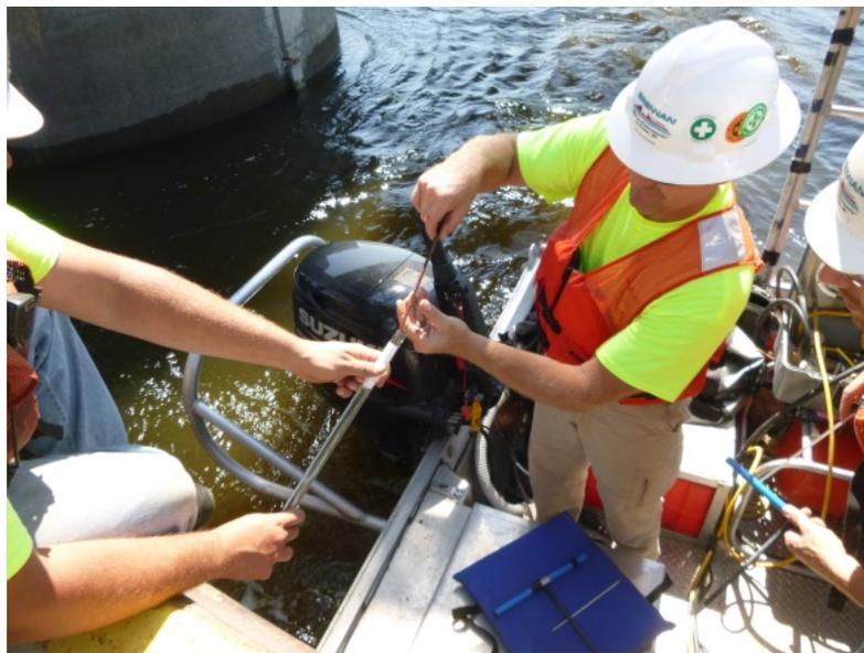
Timber Piling Cores from existing Bridge No. 5900
