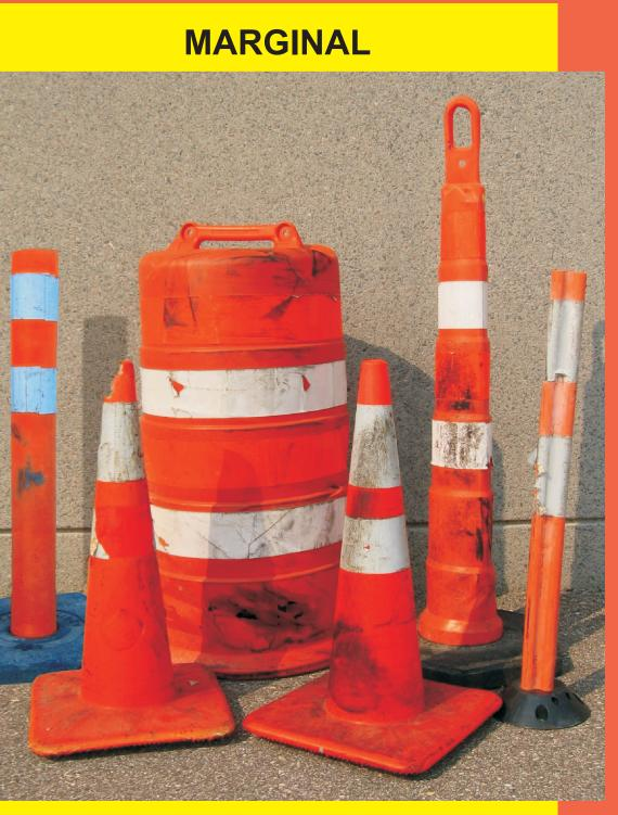
**Channelizing devices in marginal condition shall** not be installed in work zones with an anticipated duration of greater than 12 hours.
