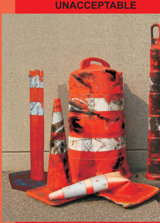
Any channelizing device that becomes unacceptable shall be replaced within 12 hours.
