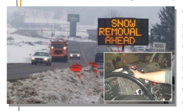
To address the concerns of the Mn/DOT snow plow operators, we equipped four of our snow plows with portable transmitters. The CMS boards are programmed to receive a signal from the transmitters any time the snow plows enter the area. When the transmitter is activated, the message on both CMS boards switches to "SNOW REMOVAL AHEAD – DRIVE WITH CAUTION."
