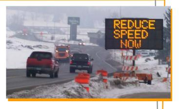
remain blank. However, if the vehicles exceed the threshold speed, the CMS flashes a two frame message that reads, "SPEED LIMIT EXCEEDED – REDUCE SPEED NOW." Response to these safety messages has been extraordinary. We have noted that out-of-town truckers exhibit the greatest response to the flashing message.
