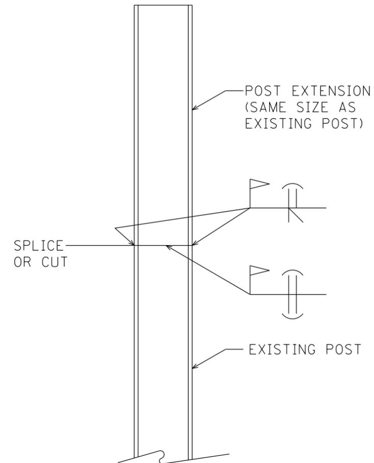
1. POST EXTENSIONS SHALL CONFORM TO MN/DOT 3306 AND SHALL BE GALVANIZED IN ACCORDANCE WITH MN/DOT 3394.
