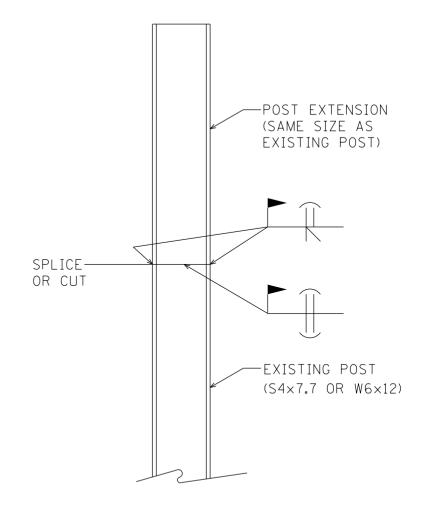
WELDED OPTION IS REQUIRED FOR EXTENSION GREATER THAN 3'-0"
