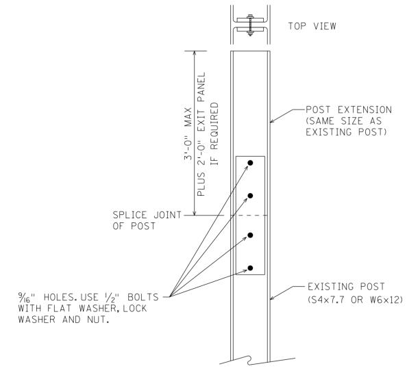
PANEL MOUNTING POST SPLICE PLATE REQUIRED ON EACH SIDE OF WEB PER EXTENSION (P 3/8" × 3" × 18")
