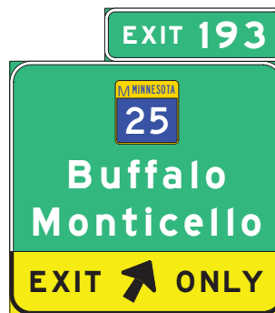
Interchange Exit Direction Lane Drop Guide Sign Type OH
