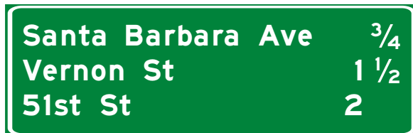
Figure 2E-31. Interchange Sequence Sign
