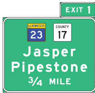
Interchange Advance Guide Sign Type A
