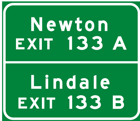
Figure 2E-24. Supplemental Guide Signs for a Multi-Exit Interchange
