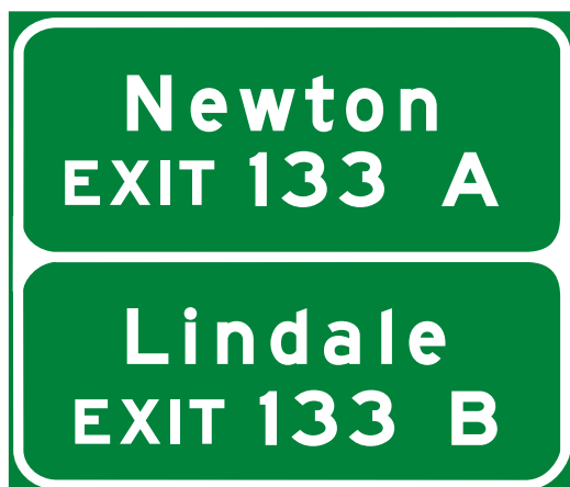
Figure 2E-17. Supplemental Guide Signs for Multi-exit Interchanges
