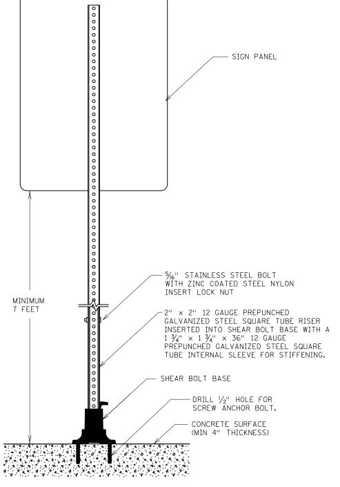
SHEAR BOLT BASE MOUNTED TO CONCRETE SURFACE
