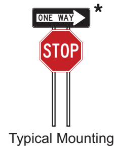
Figure 2B-17. ONE WAY Signing for Divided Highways with Median Widths Narrower Than 30 Feet and Separated Left-Turn Lanes
