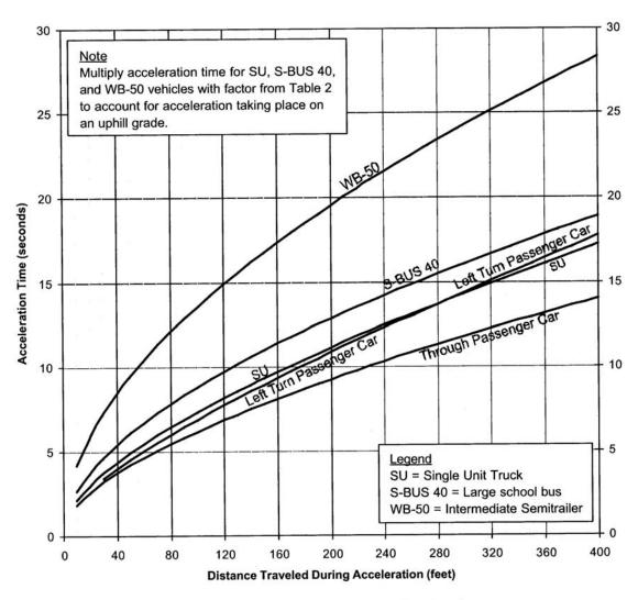
Figure 2 Acceleration time over a fixed distance on a level surface.
