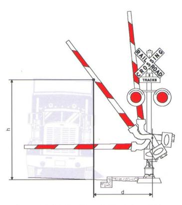
Figure 4 Gate interaction with the design vehicle.
