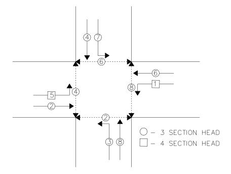
In this sequence phases 1 & 5 will be 4 section heads. The 4<sup>th</sup> section will be an additional yellow arrow that will be controlled by an overlap associated with the opposing through movement. The following is the configuration of the head with the cabinet inputs that would control each indication.
