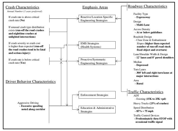
FIGURE 5 Flow Chart for Corridor Case Example
