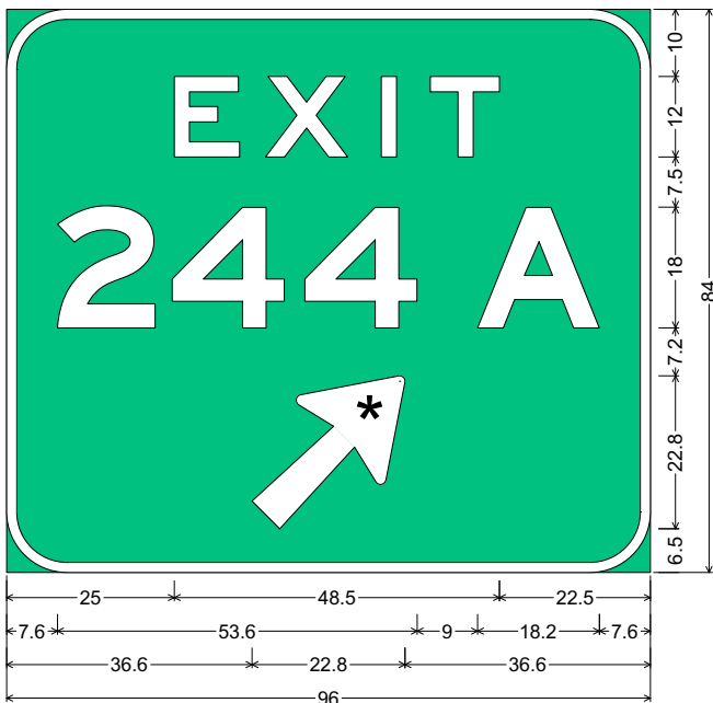
EXIT 244A 45 DEG ARROW; 9.0" Radius, 1.5" Border, White on, Green; "EXIT", F 2K specified length; "244 A", E Mod 2K; Arrow 16 - 29.0" 45';
