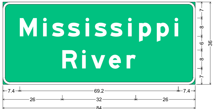
3.0" Radius, 1.0" Border, White on, Green; "Mississippi", E Mod 2K; "River", E Mod 2K;
