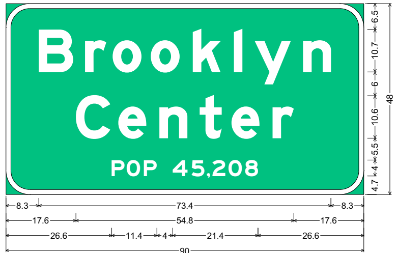
BROOKLYN CENTER POP 45,208; 1.3" Border, White on, Green; "Brooklyn", E Mod 2K; "Center", E Mod 2K; "POP", E Mod 2K; "45,208", E Mod 2K;
