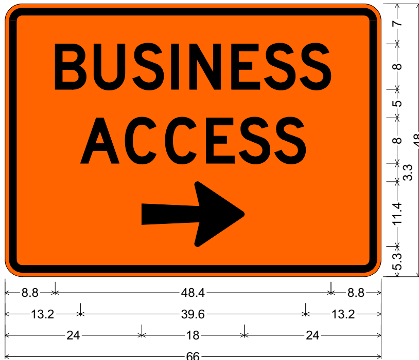
BUSINESS ACCESS RT ARROW; 3.0" Radius, 1.3" Border, 0.8" Indent, Black on Orange; "BUSINESS", D 2K; "ACCESS", D 2K; Arrow 14 - 18.0" 0';
