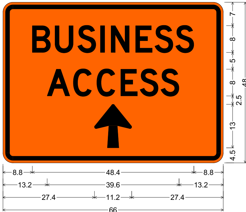
BUSINESS ACCESS UP ARROW; 3.0" Radius, 1.3" Border, 0.8" Indent, Black on Orange; "BUSINESS", D 2K; "ACCESS", D 2K; Arrow 5 - 13.0" 90';
